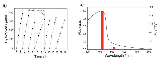
Fig. 3 (a) Plot showing sacrificial photocatalytic hydrogen evolution *versus* time for P38 under visible light irradiation ( $\lambda > 420 \text{ nm}$ , 300 W Xe light source). The vertical dashed lines indicate degassing; (b) absorption spectrum and external quantum efficiency (EQE) measured with monochromatic light in a water/MeOH/TEA mixture for P38.
