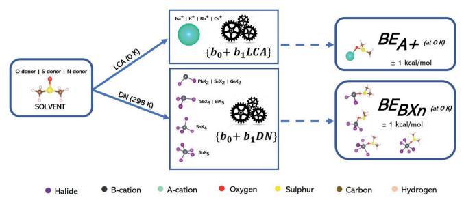
Fig. 5 Work flow showing how linear models ( $b_0 + b_1 DN/LCA$ ) describing how the affinity metrics are used to estimate the binding enthalpies of S, N, and O-donor solvents towards  $BX_n$  and  $A^+$  ions using DN and LCA values as inputs. Color code as given below the schematic. See Table 3 for the accuracy determined for each model.
