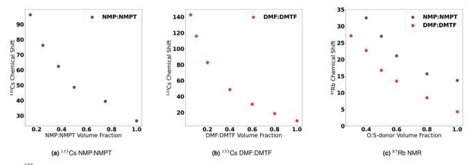
Fig. 7 133Cs NMR chemical shifts as a function of the ratio of O-donor solvent to S-donor solvent in solution showing (a) results for various mixtures of NMP and NMPT and (b) results for mixtures of DMF and DMTF. (c) 87Rb NMR chemical shifts as a function of the ratio of O-donor solvent to S-donor solvent in solution for mixtures of NMP: NMPT and DMF: DMTF.
