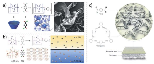
Fig. 9 (a)  $\beta$ -CD films made by interfacial polymerization from  $\beta$ -CD.<sup>153</sup> (b) Interfacial polymerization of amino-functionalized CD for TFN membrane formation.<sup>154</sup> (c) Interfacial polymerization of trianglamine with TPC for membrane formation.<sup>156</sup> Reproduced with permission from Wiley-VCH, Copyright 2017, Wiley-VCH, Copyright 2020, and Springer Nature, Copyright 2020.
