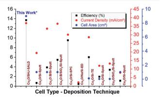
Fig. 5 Comparative study of the area, efficiency, and current density of the SALD  $Cu_2O/SHJ$  structure compared to SHJ in the literature. The compared deposition techniques are: Sputt: sputtering,  $^{39,60,61}$  SPC: spin coating,  $^{40}$  ED: electro-deposition,  $^{64}$  TE: thermally oxidized,  $^{63}$  SALD: spatial atomic layer deposition.
