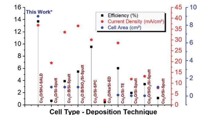
Fig. 5 Comparative study of the area, efficiency, and current density of the SALD Cu<sub>2</sub>O/SHJ structure compared to SHJ in the literature. The compared deposition techniques are: Sputt: sputtering,<sup>39,60,61</sup> SPC: spin coating,<sup>40</sup> ED: electro-deposition,<sup>64</sup> TE: thermally oxidized,<sup>63</sup> SALD: spatial atomic layer deposition.
