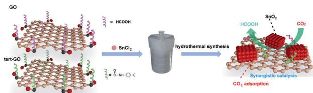
Fig. 1 Synthesis scheme of  $\text{SnO}_2/\text{GO}$  and  $\text{SnO}_2/\text{tert-GO}$ .
