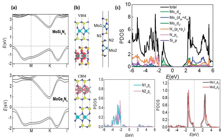
Fig. 2 (a) Band structures of bilayer MoSi<sub>2</sub>N<sub>4</sub> and MoGe<sub>2</sub>N<sub>4</sub>. (b) Distributions of valence band maximum (VBM) and conduction band minimum (CBM) bands, and (c) PDOS analysis for bilayer MoSi<sub>2</sub>N<sub>4</sub>.
