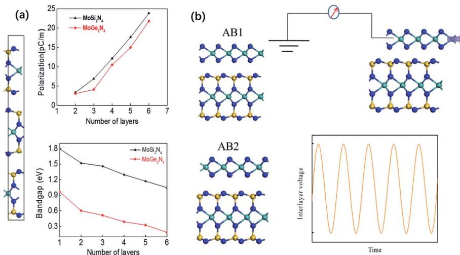
Fig. 4 (a) The dependences of polarizations and bandgaps of ABC stacking MoSi<sub>2</sub>N<sub>4</sub> and MoGe<sub>2</sub>N<sub>4</sub> thin-layers on the thickness. (b) Different stacking configurations of MoN<sub>2</sub>/MoSi<sub>2</sub>N<sub>4</sub> hetero-bilayer with distinct interlayer potentials, which can be utilized as nanogenerators.
