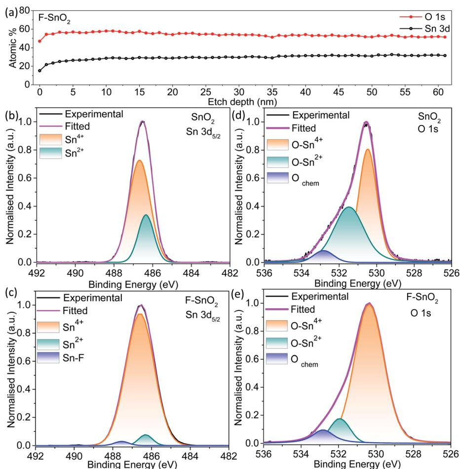
Fig. 3 (a) Atomic percentages of Sn 3d and O 1s calculated from XPS of the F-SnO<sub>2</sub> film at different depths. Deconvoluted XPS spectra of (b and c) Sn 3d<sub>5/2</sub> and (d and e) O 1s of pristine SnO<sub>2</sub> and F-SnO<sub>2</sub>, respectively.
