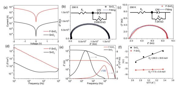
Fig. 4 (a) I-V characteristics and (b and c) Nyquist plots of SnO<sub>2</sub> and F-SnO<sub>2</sub> films, respectively. Inset in (b and c) shows the equivalent circuit diagram used for fitting. (d) Capacitance *versus* frequency. (e) Real part (Z') and imaginary part (-Z'') of impedance as a function of frequency for SnO<sub>2</sub> and F-SnO<sub>2</sub> films. (f) Arrhenius plot of ln( $\tau$ ) *versus* 1/T ( $K^{-1}$ ) obtained from impedance analysis at different temperatures.
