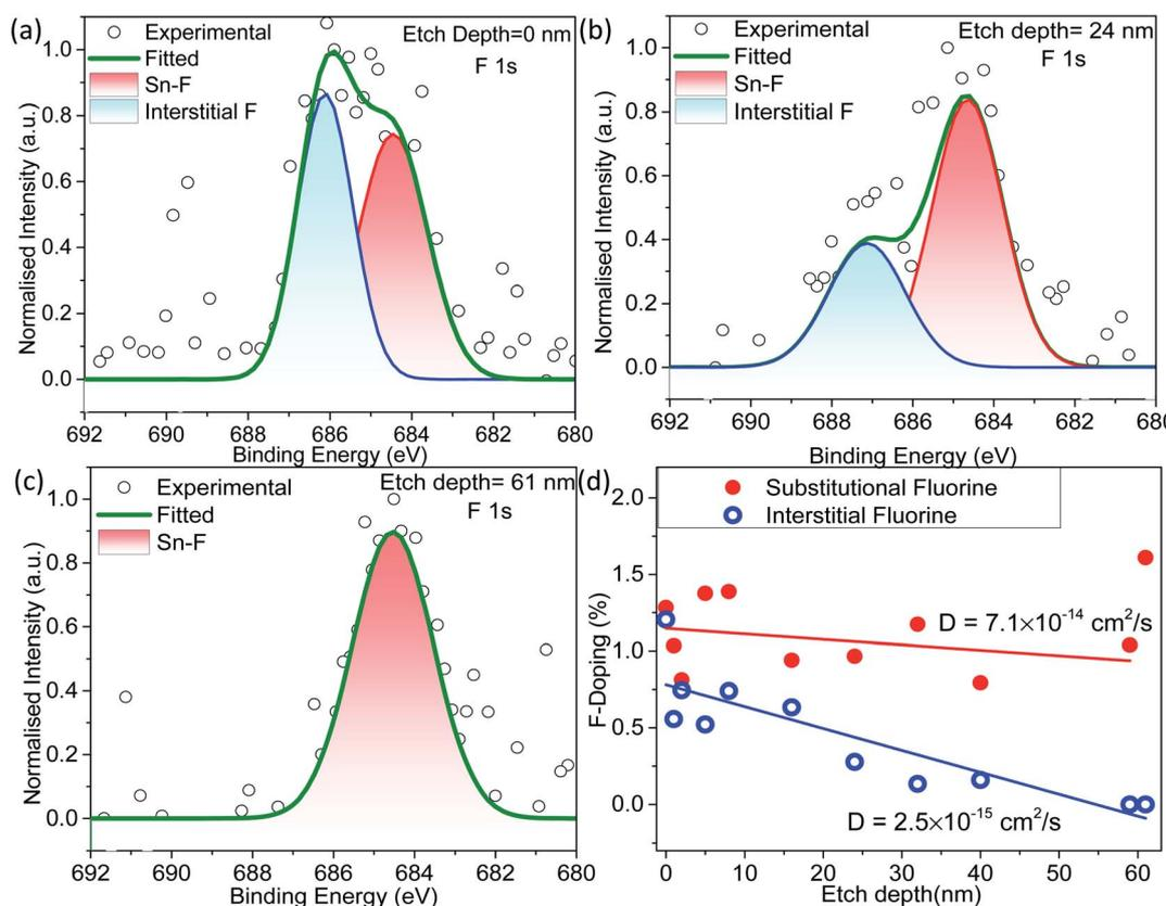
Fig. 2 Deconvoluted XPS spectra of F 1s from different etching depths of (a) 0 nm (at the surface), (b) 24 nm, and (c) 61 nm of F- $\text{SnO}_2$ , respectively. Spectra (a–c) are normalized to the maximum intensity. (d) Variation in substitutional and interstitial fluorine percentage present in the F- $\text{SnO}_2$  lattice.
