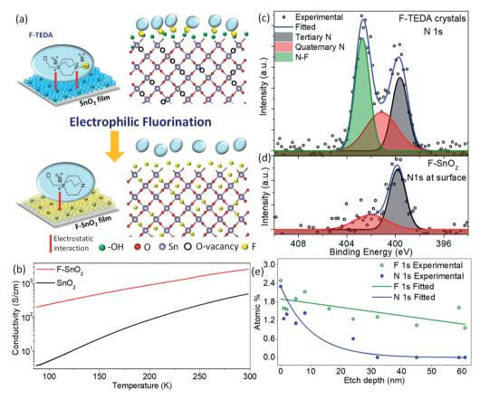
Fig. 1 (a) Schematic demonstrating the fluorination process of the SnO<sub>2</sub> film using the F-TEDA molecule as the fluorinating precursor. (b) Temperature-dependent conductivity of SnO2 and F-SnO2 films. (c and d) Deconvoluted N 1s HR-XPS spectra of the F-TEDA precursor compared with the F-SnO<sub>2</sub> film. (e) Atomic % distribution versus etch depth for N 1s and F 1s across the F-SnO<sub>2</sub> film.
