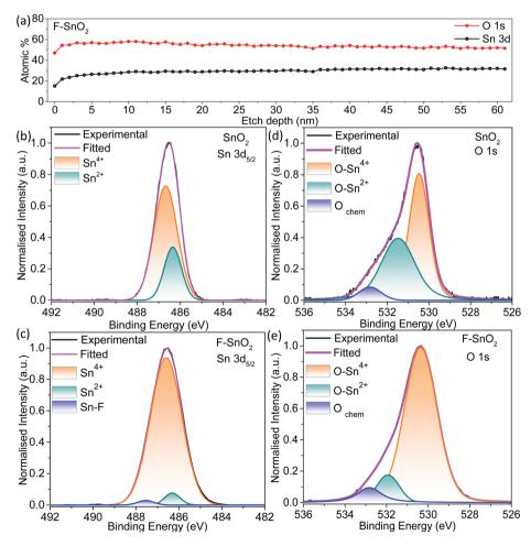
Fig. 3 (a) Atomic percentages of Sn 3d and O 1s calculated from XPS of the F-SnO<sub>2</sub> film at different depths. Deconvoluted XPS spectra of (b and c) Sn 3d<sub>5/2</sub> and (d and e) O 1s of pristine SnO<sub>2</sub> and F-SnO<sub>2</sub>, respectively.
