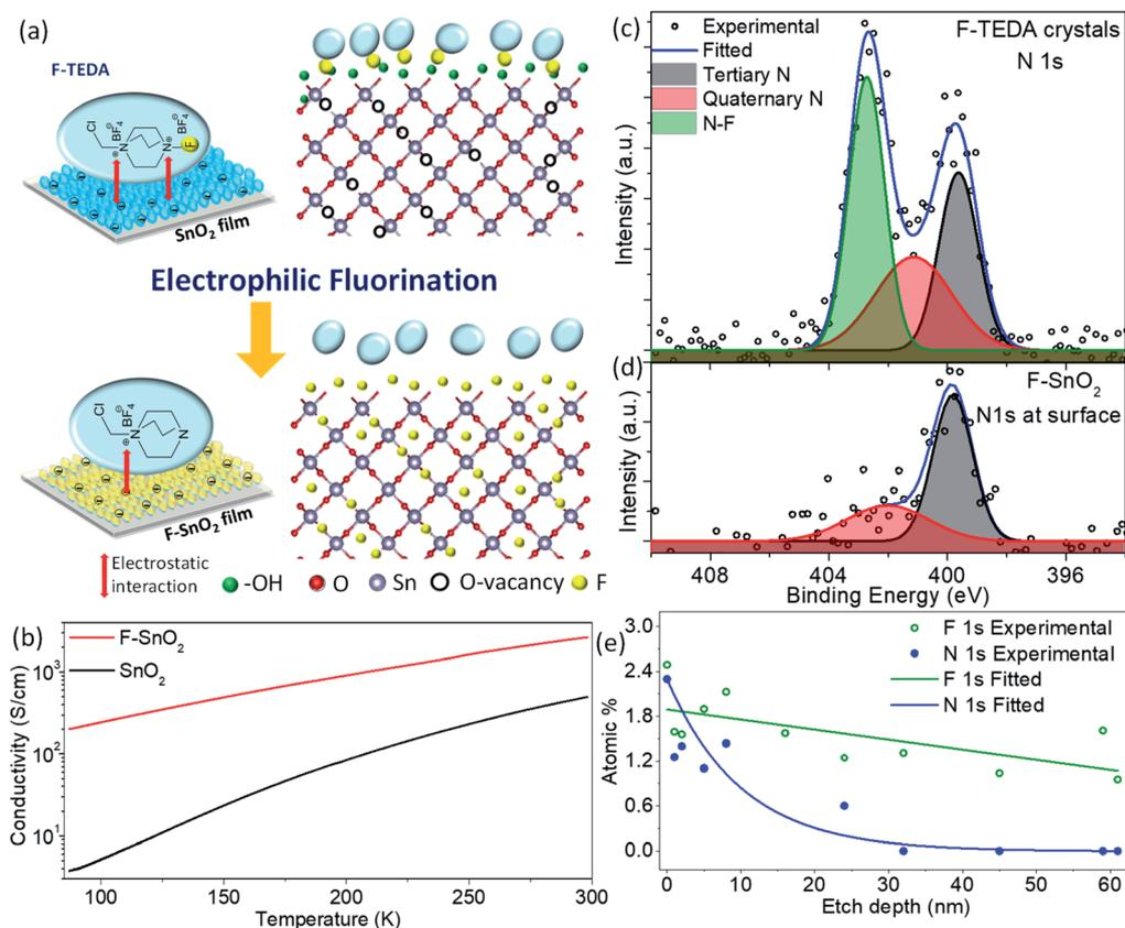
Fig. 1 (a) Schematic demonstrating the fluorination process of the  $\text{SnO}_2$  film using the F-TEDA molecule as the fluorinating precursor. (b) Temperature-dependent conductivity of  $\text{SnO}_2$  and F- $\text{SnO}_2$  films. (c and d) Deconvoluted N 1s HR-XPS spectra of the F-TEDA precursor compared with the F- $\text{SnO}_2$  film. (e) Atomic % distribution versus etch depth for N 1s and F 1s across the F- $\text{SnO}_2$  film.
