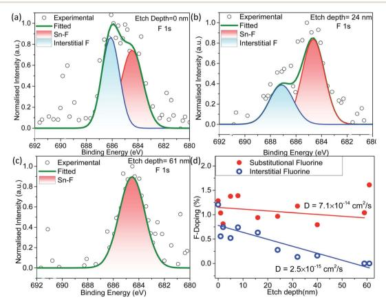
Fig. 2 Deconvoluted XPS spectra of F 1s from different etching depths of (a) 0 nm (at the surface), (b) 24 nm, and (c) 61 nm of  $F-SnO_2$ , respectively. Spectra (a–c) are normalized to the maximum intensity. (d) Variation in substitutional and interstitial fluorine percentage present in the  $F-SnO_2$  lattice.
