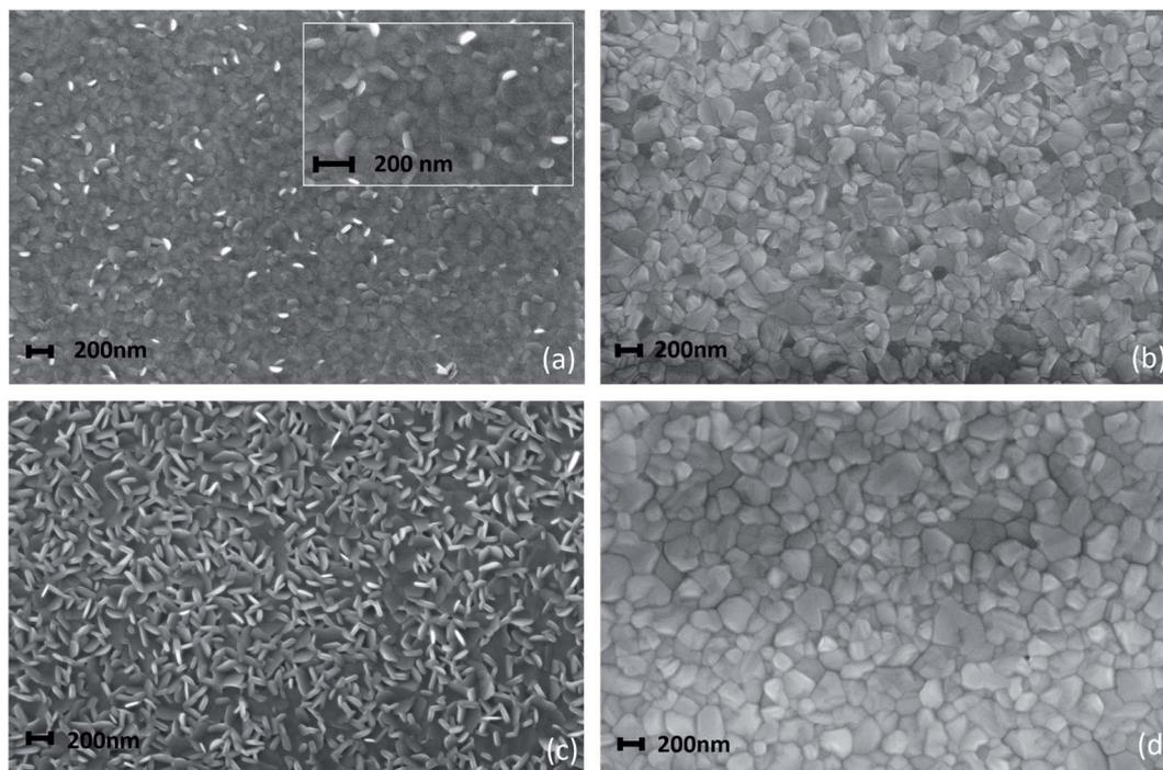
Fig. 6 SEM images collected on (a)  $\text{PbI}_2$  deposited on an ITO/PTAA substrate using a deposition time of 15 minutes and (b) the converted  $\text{MAPbI}_3$  after 30 minutes of MAI deposition. (c)  $\text{PbI}_2$  deposited for 30 minutes and (d) the resultant  $\text{MAPbI}_3$  after 60 minutes of MAI deposition.
