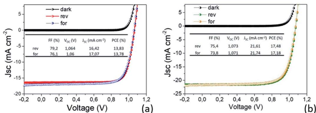
Fig. 9  $I$ - $V$  characterization of the best prepared devices with (a) 80 nm and (b) 150 nm MAPbI<sub>3</sub> active layers. The AVT moves from 32.8% to 20%.
