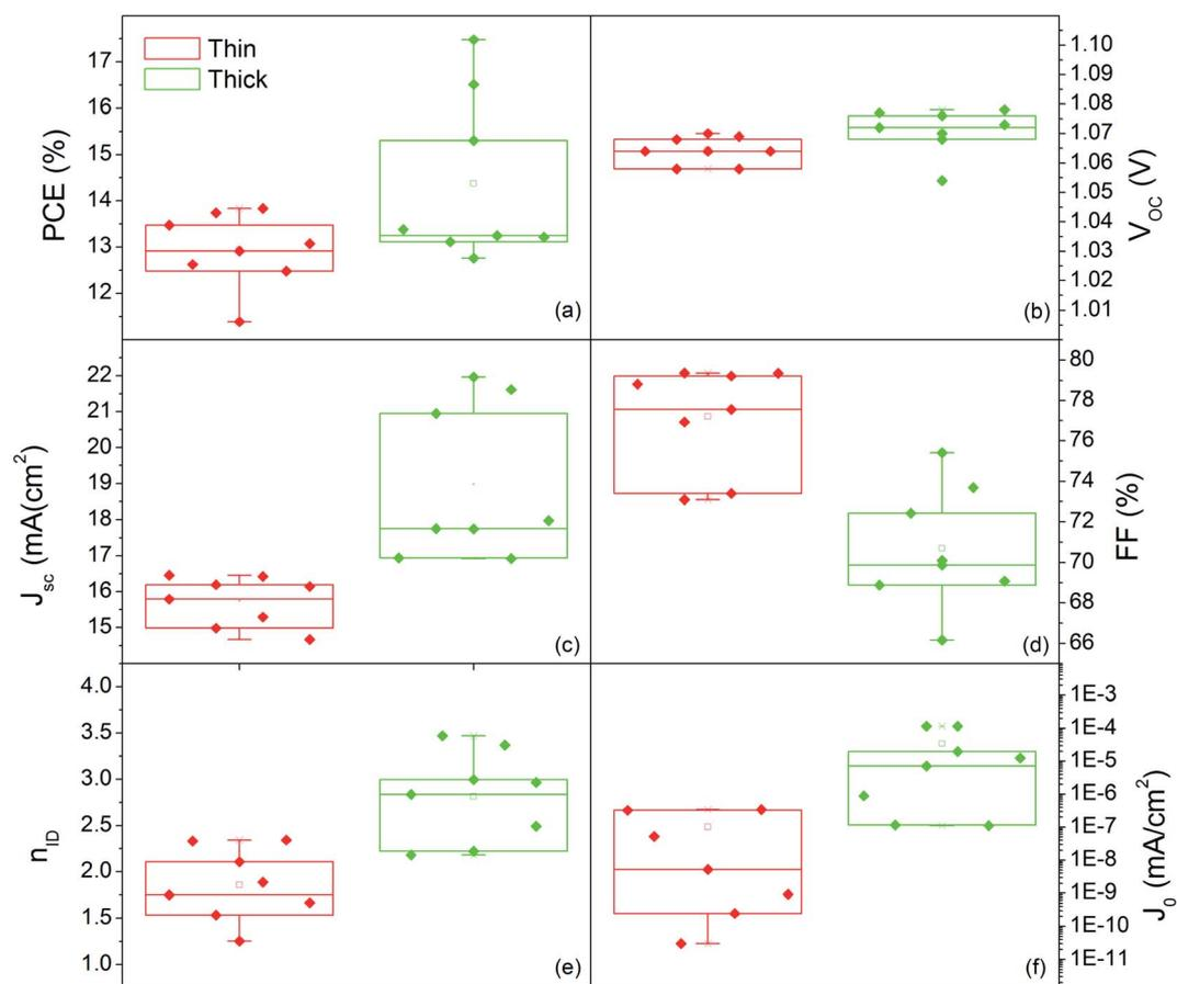
Fig. 10 Box plot of (a) efficiency (PCE), (b) open circuit voltage (*V*<sub>oc</sub>), (c) short circuit current (*J*<sub>sc</sub>), (d) fill factor (FF), (e) ideality factor (*n*<sub>ID</sub>) and (f) reverse saturation current (*J*<sub>0</sub>) from the electrical characterization of all the prepared devices with 80 nm thick and 150 nm thick MAPbI<sub>3</sub> active layers.
