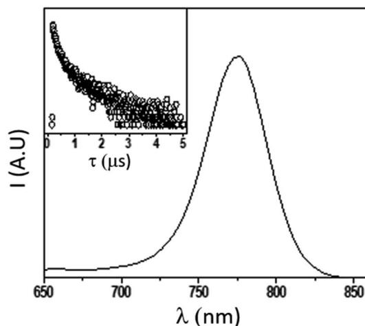
Fig. 8 Emission spectrum (main, exc = 405 nm) and corresponding lifetime decay (inset, exc = 405 nm; em: 750 nm) of MAPbI<sub>3</sub> thin film on glass.
