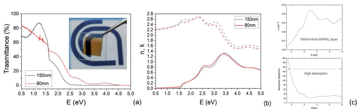
Fig. 7 (a) Transmittances of 150 nm and 80 nm  $\text{MAPbI}_3$  films. (b) The refractive index  $n$  (dashed line) and the extinction coefficient  $k$  (solid line) of 150 nm and 80 nm  $\text{MAPbI}_3$  films. Note the pre-gap tail that is close to ideality in the 150 nm-thick layer. (c) Absorption coefficient ( $\text{nm}^{-1}$ ) and absorption depth (nm) of 150 nm-thick  $\text{MAPbI}_3$  layers.
