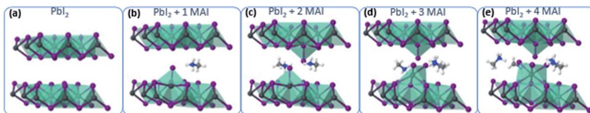
Fig. 4 DFT calculations of MAI intercalation within  $\text{PbI}_2$  layers. (a) Ideal  $\text{PbI}_2$  structure and intercalation of (b) 1 MAI molecule, (c) 2 MAI molecules, (d) 3 MAI molecules and (e) 4 MAI molecules within the layers of the  $\text{PbI}_2$  structure.
