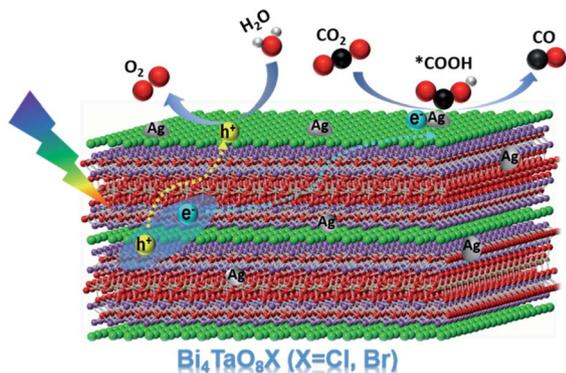
Scheme 1 The proposed mechanism of photocatalytic CO<sub>2</sub> reduction to CO on Bi<sub>4</sub>TaO<sub>8</sub>X.
