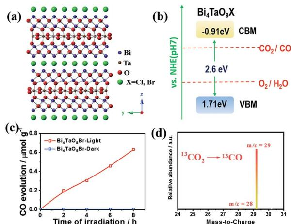
Fig. 1 (a) The crystal structure of Bi<sub>4</sub>TaO<sub>8</sub>X (X = Cl, Br). (b) A schematic illustration of the band structure of Bi<sub>4</sub>TaO<sub>8</sub>X (X = Cl, Br). (c) The time course of photocatalytic CO<sub>2</sub> reduction on Bi<sub>4</sub>TaO<sub>8</sub>Br. (d) GC-MS analysis of the generated CO using <sup>13</sup>CO<sub>2</sub> as the feedstock.
