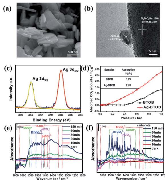
**Fig. 4** (a and b) SEM and HRTEM image of Bi<sub>4</sub>TaO<sub>8</sub>Br-F loaded with Ag. (c) The XPS fine spectrum of silver in Ag-Bi<sub>4</sub>TaO<sub>8</sub>Br-F. (d) The absorption curves of CO<sub>2</sub> on Bi<sub>4</sub>TaO<sub>8</sub>Br-F and Ag-Bi<sub>4</sub>TaO<sub>8</sub>Br-F at room temperature. (e and f) *In situ* FTIR spectra of photocatalytic CO<sub>2</sub> reduction on Bi<sub>4</sub>TaO<sub>8</sub>Br-F and Ag-Bi<sub>4</sub>TaO<sub>8</sub>Br-F.
