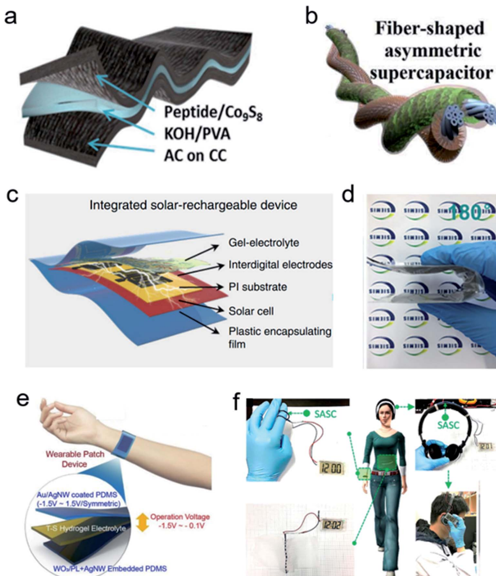
Fig. 7 (a) Schematic illustration of a flexible solid-state ASC. 74 Copyright 2019, Elsevier. (b) The schematic diagram of a fiber-shaped ASC device. 75 Copyright 2018, Elsevier. (c) Schematic illustration of an integrated solar-charging self-powered unit, and (d) digital photo showing its bending condition. 76 Copyright 2019, Springer Nature. (e) Schematic illustration of a wearable patch device based on transparent ASCs. 77 Copyright 2019, American Chemical Society. (f) A view of application of fiber-shaped ASCs in various electronic devices, including a watch, headphone and lab cloth. 78 Copyright 2018, American Chemical Society.
