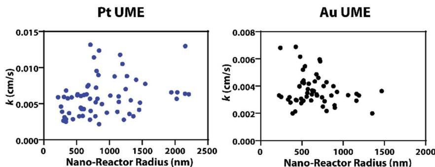
Fig. 2 Plots demonstrating the effect that aqueous nanodroplet size, filled with 50 mM CuCl<sub>2</sub> and glycerol (50%, v/v), has on the heterogeneous rate kinetics on a Pt and Au microelectrode. The large spread in the data without an observed trend indicates they are independent of nanodroplet size.
