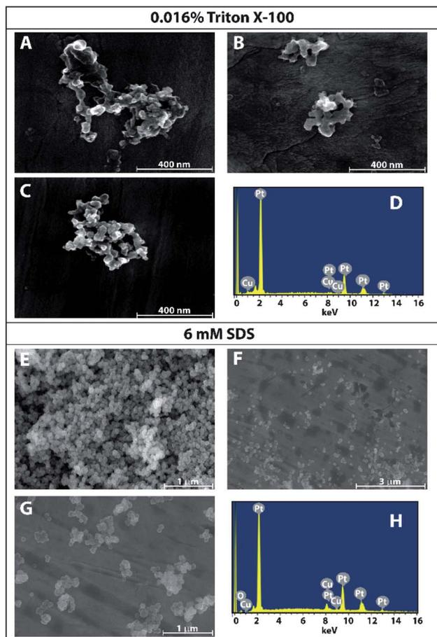
Fig. 3 SEM images and representative EDX spectra showing the morphologies of copper nanoparticles (NPs) deposited on platinum foil from aqueous nanodroplets containing 50 mM  $\text{CuCl}_2$  with added surfactants in a continuous phase of 0.1 M  $[\text{TBA}][\text{PF}_6]$  in 1,2-DCE. (A–D) SEM data and corresponding EDX using an added surfactant of 0.016% w/v Triton X-100. (E–H) SEM data using an added surfactant of 6 mM SDS ( $r = 28 \text{ nm} \pm 11 \text{ nm}$ ).
