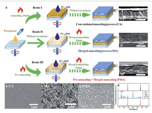
Fig. 1 (a) Schematic illustration of three fabrication processes for a  $PC_{61}BM$  coated (3AMP)(MA $_{0.75}FA_{0.25}$ )<sub>3</sub>Pb<sub>4</sub>I $_{13}$  film and the cross-sectional SEM images for the corresponding films. Top-view SEM images of (3AMP)(MA<sub>0.75</sub>FA<sub>0.25</sub>)<sub>3</sub>Pb<sub>4</sub>I<sub>13</sub> films fabricated by CA (b), MA (c) and PMA (d) processes. (e) X-ray diffraction (XRD) patterns of perovskite films fabricated by various methods.
