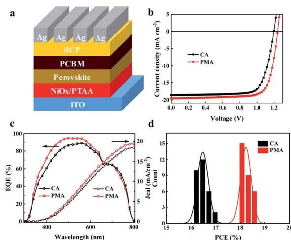
Fig. 2 Planar structured PVSC device configuration (a), *J*–*V* curves (b), EQE spectra and the integrated photocurrent curves (c) of the CA and PMA based devices, and PCE histogram of 30 devices fabricated by the CA or PMA process (d).
