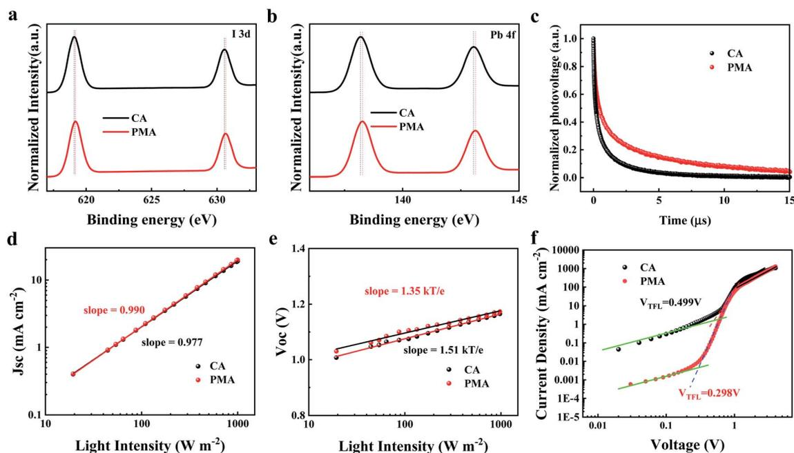
Fig. 4 | I 3d core level (a), Pb 4f core level (b) XPS spectra of the CA- and PMA-based perovskite films with the PC<sub>61</sub>BM layer rinsed away. (c) TPV decay curves of the devices fabricated by CA and PMA processes. Measured  $J_{sc}$  (d),  $V_{oc}$  (e) of CA- and PMA-based devices plotted against light intensity (dots), together with linear fits (solid lines) to the data. (f)  $J$ - $V$  curves of the electron-only devices fabricated by CA and PMA processes.
