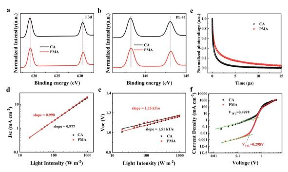
Fig. 4 I 3d core level (a), Pb 4f core level (b) XPS spectra of the CA- and PMA-based perovskite films with the PC<sub>61</sub>BM layer rinsed away. (c) TPV decay curves of the devices fabricated by CA and PMA processes. Measured  $J_{\rm sc}$  (d),  $V_{\rm oc}$  (e) of CA- and PMA-based devices plotted against light intensity (dots), together with linear fits (solid lines) to the data. (f) J-V curves of the electron-only devices fabricated by CA and PMA processes.
