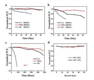
Fig. 5 Stability measurements: (a) at room temperature with humidity  $25 \pm 5\%$ , (b) at room temperature with humidity of  $45 \pm 5\%$ , (c) at  $85 \,^{\circ}$ C in an N<sub>2</sub>-filled glovebox for the 3D and 2D PVSCs. (d) Thermal-cycling test for the PMA-based device
