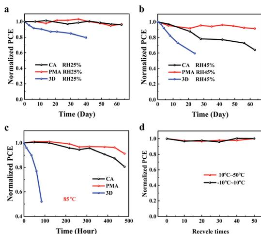
Fig. 5 Stability measurements: (a) at room temperature with humidity  $25 \pm 5\%$ , (b) at room temperature with humidity of  $45 \pm 5\%$ , (c) at  $85 \text{ }^\circ\text{C}$  in an  $\text{N}_2$ -filled glovebox for the 3D and 2D PVSCs. (d) Thermal-cycling test for the PMA-based device.
