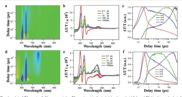
Fig. 3 2D color plot of TA spectra (left), representative TA spectra at indicated delay times (middle), and TA kinetics probed at different-n perovskite bands (right) obtained by irradiating the perovskite films using a 365 nm laser with a fluence below  $1\,\mu\text{J}$  cm $^{-2}$  from the back (glass). (a– c) Device fabricated by CA, (d-f) device fabricated by PMA.
