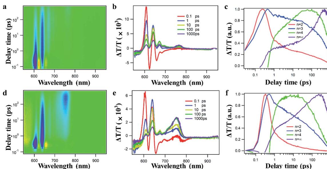
Fig. 3 2D color plot of TA spectra (left), representative TA spectra at indicated delay times (middle), and TA kinetics probed at different- $n$  perovskite bands (right) obtained by irradiating the perovskite films using a 365 nm laser with a fluence below  $1 \mu\text{J cm}^{-2}$  from the back (glass). (a–c) Device fabricated by CA, (d–f) device fabricated by PMA.
