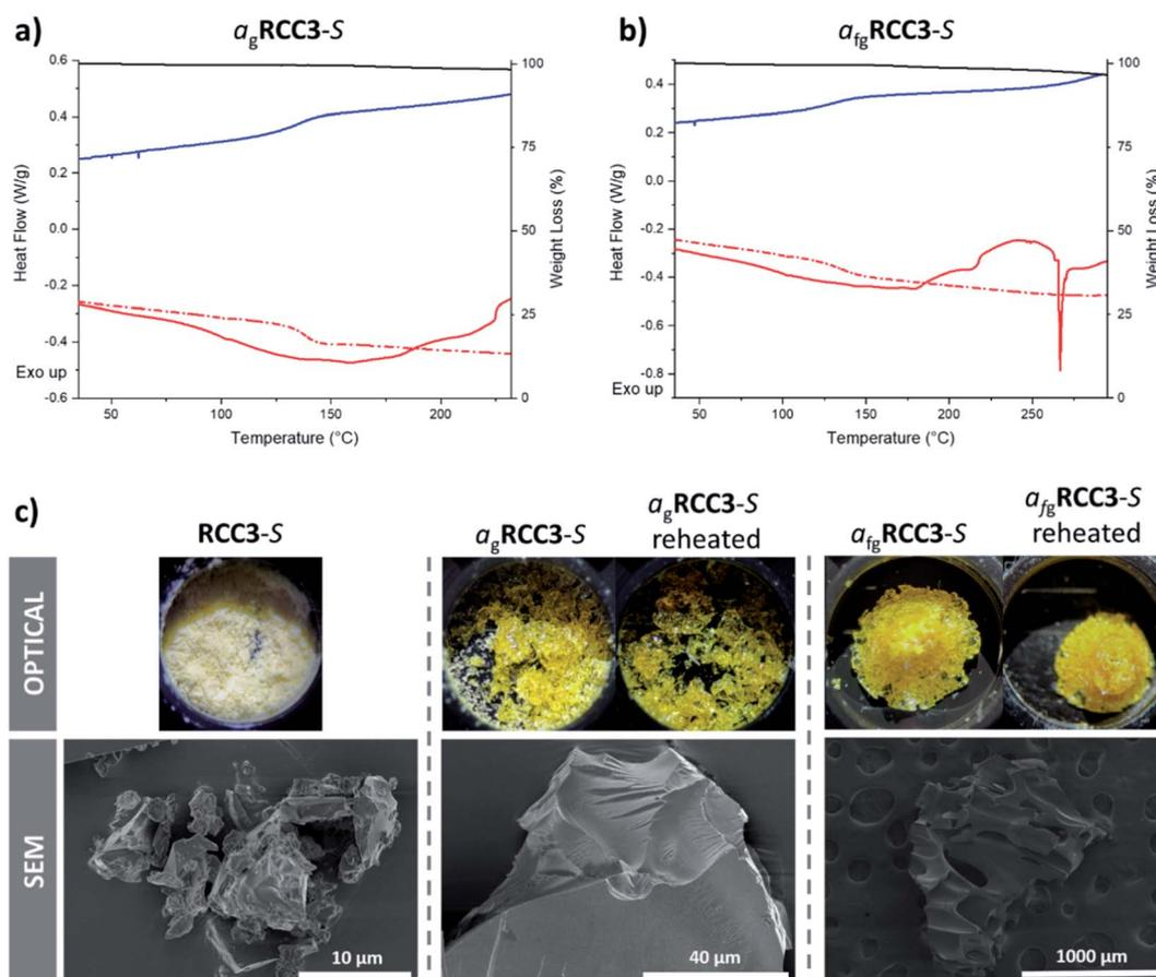
Fig. 2 DSC traces and corresponding TGA curve (black) of **RCC3-S** subjected to heat–cool–heat (HCH) cycles to (a) 250 °C forming  $a_g$ RCC3-S, and (b) 300 °C forming  $a_{fg}$ RCC3-S. DSC traces: initial upscan shown as a solid red line, downscan as a blue line, and second upscan as a dashed red line. Optical and SEM images of **RCC3-S**,  $a_g$ RCC3-S, and  $a_{fg}$ RCC3-S (c).
