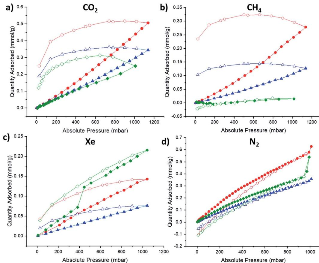
Fig. 5 Adsorption (filled) and desorption (empty) isotherms for RCC3-S (green),  $a_g$ RCC3-S (red),  $a_{fg}$ RCC3-S (blue): (a) CO<sub>2</sub>, 273 K; (b) CH<sub>4</sub>, 273 K; (c) Xe, 273 K; (d) N<sub>2</sub>, 77 K.
