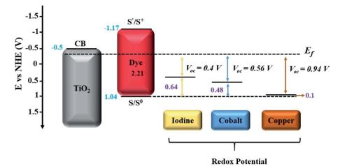
Energetics in DSSCs with respect to redox potentials of each redox couple  $(|-/|_3^-, [Co(bpy)_3]^{2+/3+}$  and  $[Cu(dmp)_2]^{1+/2+})$  utilized in DSSCs.<sup>55</sup>
