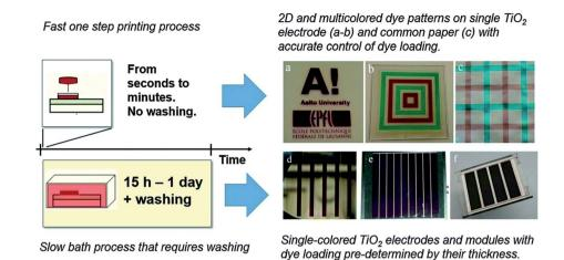
Fig. 7 Rapidly sensitized photoelectrodes *via* inkjet printed dyes accelerates the staining process and can also be adopted to produce multi-colour printed dyes based TiO<sub>2</sub> electrodes and for precise co-sensitization of the PEs (reproduced from ref. 31 with permission).
