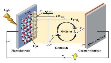
Fig. 2 Schematic illustration representing device structure and working principle of a dye-sensitized solar cell. CB = conduction band,  $E_{f TiO2}$  = fermi level of TiO<sub>2</sub>, S = ground state of dye sensitizer molecule, S\* = excited state of dye sensitizer molecule, S<sup>0</sup> = oxidized dye, S<sup>+</sup> = charge separation, I<sup>-</sup> = iodide ion and I<sub>3</sub><sup>-</sup> = triiodide ion.
