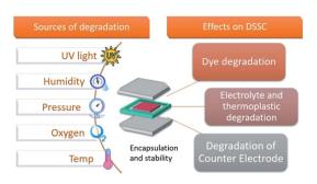
Fig. 9 Illustration of the factors that affect DSSC devices and their possible consequences which hinder the photovoltaic performance.
