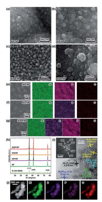
Fig. 2 Morphological and structural characterization of the asprepared electrodes: SEM images for (a) NiP/NF, (b) NiS/NF, and NiSP/ NF at (c) low and (d) high magnifications. SEM/EDX elemental mappings for (e) NiP/NF, (f) NiS/NF, and (g) NiSP/NF. (h) XRD results. (i) HRTEM image of NiSP/NF. The inset displays the corresponding SAED pattern. (j) TEM/EDX elemental mappings for NiSP/NF.
