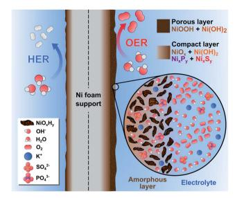
Fig. 7 Schematic illustration of the dynamic reconstruction process occurred during the HER and the OER on the NiSP electrocatalytic
