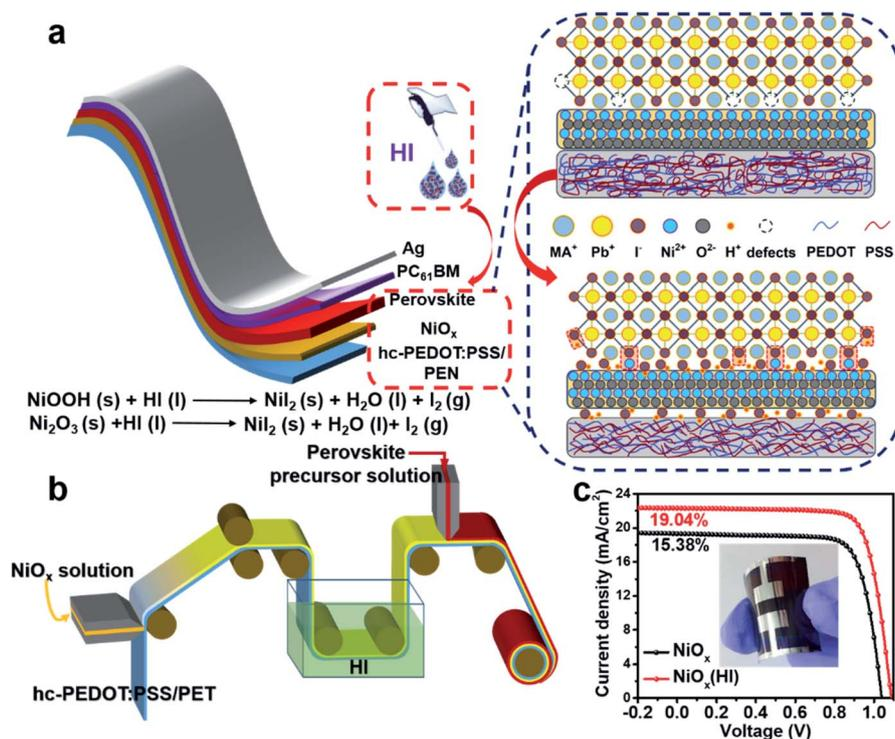
Fig. 1 *In situ* bifacial passivation mechanism and device preparation. (a) Diagram of the passivation mechanism. (b) Fabrication procedure for perovskite solar cells by R2R process. (c) *J*-*V* curves of flexible devices (1.01 cm<sup>2</sup>) with and without HI treatment. Inset presents the photograph of flexible perovskite solar cells.
