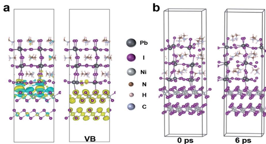
Fig. 3 The Interface interaction between  $\text{NiO}_x$  (HI) and perovskite films. (a) Charge differential density analysis of the interfaces. (b) *Ab initio* molecular dynamics (AIMD) of the interaction between  $\text{NiI}_2$  and perovskite. For simplifying the calculation,  $\text{MAPbI}_3$  perovskite supercell is used for AIMD simulation.
