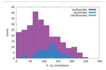
Fig. 6 Distribution of the stabilization energy, defined as the lowest energy of all prototypes used minus the energy of the five-atom cell depicted in Fig. 1. The width of the bins is 20 meV per atom.
