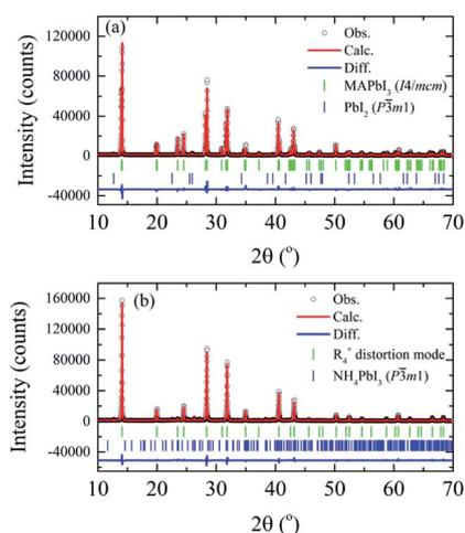
Fig. 4 X-ray powder diffraction data and Rietveld refinements at room temperature of the (a) MAPbI<sub>3</sub> as-compacted sample and (b) submitted to thermal annealing at 250 °C for 40 hours.
