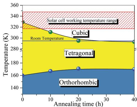
Fig. 6 Phase diagram proposed for the MAPbI<sub>3</sub> halide perovskite taking into account the observed shift in the phase transition temperature with different annealing conditions. The horizontal bar corresponds to room temperature, and the hatched region indicates the solar cell working temperature range.
