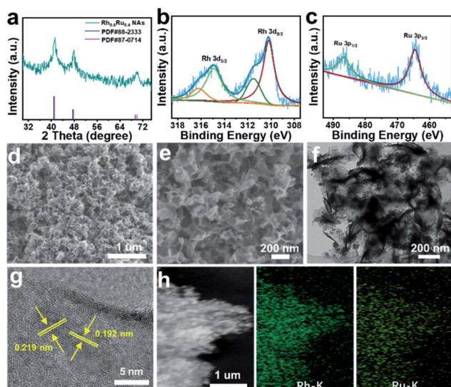
Fig. 1 (a) XRD patterns of the obtained Rh<sub>0.6</sub>Ru<sub>0.4</sub> NAs. The high-resolution XPS spectra of (b) Rh 3d and (c) Ru 3p electrons for Rh<sub>0.6</sub>Ru<sub>0.4</sub> NAs. (d) SEM image and (e) enlarged SEM image for Rh<sub>0.6</sub>Ru<sub>0.4</sub> NAs. (f) TEM image and (g) HRTEM image taken from Rh<sub>0.6</sub>Ru<sub>0.4</sub> NAs. (h) SEM image and corresponding EDX elemental mapping images for Rh<sub>0.6</sub>Ru<sub>0.4</sub> NAs.
