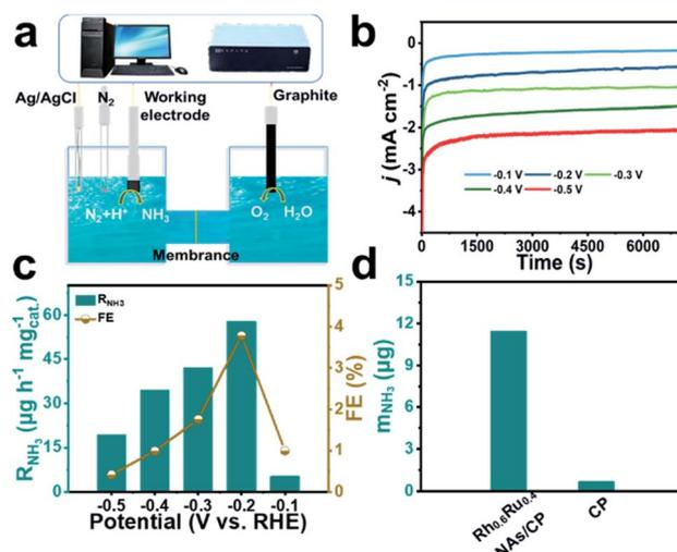
Fig. 2 (a) Schematic diagram depicting the electrocatalytic setup for the eNRR test. (b) Chronoamperometry tests of Rh<sub>0.6</sub>Ru<sub>0.4</sub> NAs/CP for the eNRR at different potentials. (c)  $R_{\text{NH}_3}$  and FE of Rh<sub>0.6</sub>Ru<sub>0.4</sub> NAs/CP for the eNRR test at different potentials. (d)  $m_{\text{NH}_3}$  of Rh<sub>0.6</sub>Ru<sub>0.4</sub> NAs/CP and bare CP for the eNRR test at -0.2 V (vs. RHE).
