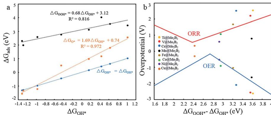
Fig. 6 (a) Scaling relationship between the  $\Delta G_{\text{OH}^*}$  and  $\Delta G_{\text{O}^*}$ ,  $\Delta G_{\text{OOH}^*}$  at site I. (b) Dual volcano plot for the OER and ORR for TM@Mo<sub>2</sub>B<sub>2</sub> at site I.
