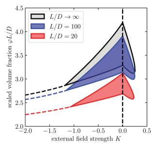
Fig. 3 Phase diagram of hard spherocylinders with aspect ratios  $L/D \in \{\infty,\ 100,\ 20\}$  in terms of a scaled volume fraction as function of the external field strength K. Within the enclosed region, high and low density phases coexist. We computed the location of the binodals using the Onsager free energy, with scaled particle theory corrections for finite particle aspect ratios. The terminology of the phases is unchanged and shown in Fig. 1.
