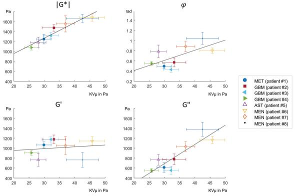
Fig. 5 Correlation analysis of viscoelastic parameters obtained by MRE in *in vivo* brain tumors and by OS in single cancer cells. MRE measured magnitude ( $|G^*|$ ), loss angle ( $\varphi$ ), real part (G') and imaginary part (G'') of the complex shear modulus  $G^*$ . OS deformations were converted to stiffness according to the Kelvin-Voigt model ( $KV\mu$ ).
