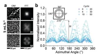
Fig. 8 Effect of oscillatory flow at 5 mL  $h^{-1}$  on  $L_{\alpha}$  phase over multiples cycles from 0-50. (a) Morphology evolution observed by cross-polarised optical microscopy at the channel wall and corresponding FFTs, associated with MLV formation; (b) oscillatory shear cycle azimuthal average of FFTs (computed within  $0.12-0.18 \mu m^{-1}$ ).
