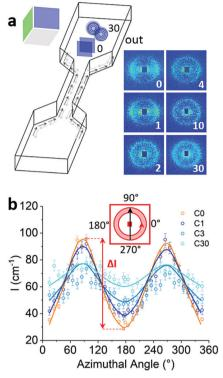
Fig. 9 Oscillatory flow SANS analysis. (a) Microfluidic SANS 2D scattering images of oscillatory shear cycles (measured at 8 m and  $\lambda$  = 6 Å); (b) azimuthal average for selected cycles 0, 1, 3 and 30 within  $0.035 \le$  $q \le 0.045 \, \text{Å}^{-1}$  computed from the 2D data shown in panel (a), from where an orientation parameter  $\Delta l$  is estimated from the difference between the maximum and minimum intensities as a function of azimuthal angle.
