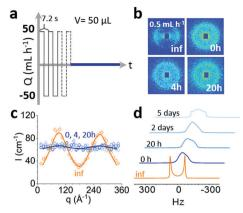
Fig. 10 MLV stability after shearing. (a) Oscillatory shear profile with flow rate of 50 mL  $h^{-1}$  and 50  $\mu$ L volume amplitude applied for 500 cycles; (b) 2D SANS scattering images collected before and 0, 4 and 20 h after cessation of shear; (c) azimuthal average within 0.035  $\leq q \leq$  0.045 Å<sup>-1</sup> computed from the 2D data shown in panel (b). (d) <sup>2</sup>H NMR relaxation over several days. Vesicles remain stable for up to 2 days
