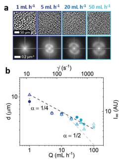
Fig. 7 MLV size dependence on flow rate. (a) Cross-polarised optical images and their corresponding FFTs at selected flow rates 1-50 mL h<sup>-1</sup>. (b) Vesicle size (°) and the asymptotic average optical image intensity ( $\Delta$ ) dependence on flow rate. Data are generally described by a 1/4 power with wall shear rate; given the data scatter, the 1/2 power (observed by Roux<sup>6</sup>) can not be ruled out above 20 s<sup>-1</sup> shear rate.
