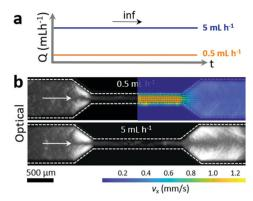
Fig. 3 Continuous flow. (a) Constant volumetric flow rate over time, illustrated here for 0.5 and 5 mL  $h^{-1}$ , corresponding to an average velocity within the constriction of  $\simeq 1.49$  and 14.9 mm s<sup>-1</sup>, respectively; (b) crosspolarised microscopy images of the fluid flow at the two flow rates with PIV for 0.5 mL h<sup>-1</sup> indicating plug-like flow.
