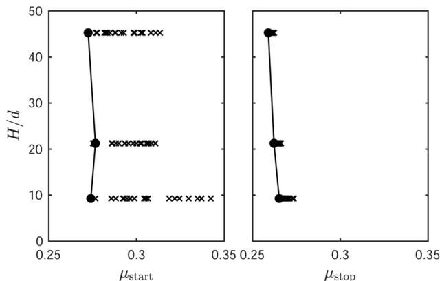
Fig. 8 Critical stresses  $\mu_{\text{start}}$  and  $\mu_{\text{stop}}$  in simple plane shear versus true system height  $H/d$ , obtained from 20 different DEM runs. The crosses show the individual transition stresses pertaining to every run, while the filled circles represent the deterministic value extracted from the linear fit of the CDF.
