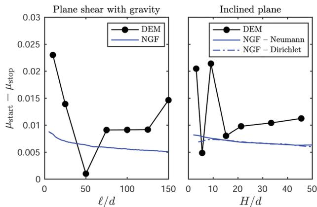
Fig. 9 Critical stress difference  $\mu_{\text{start}} - \mu_{\text{stop}}$  versus dimensionless loading length scale  $\ell/d$  for plane shear with gravity, and versus dimensionless layer height  $H/d$  for inclined plane. The DEM data (filled circles) and NGF data (blue lines) is the same as in Fig. 6(c, f) and 7(c, f).
