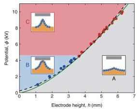
Fig. 7 Comparison of theoretical regime boundaries. The green solid line is plotted from the scaling analysis,  $\phi = \eta(\rho q/\Delta \varepsilon)^{1/2} h^{3/2}$ , by taking the prefactor  $\eta$  as 1.2. The black dotted line is the boundary obtained by egn (A3) taking  $\partial \phi / \partial H = 0$ .
