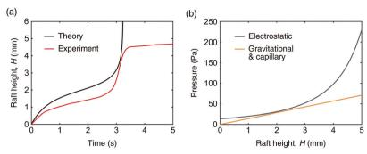
Fig. 8 The dynamics of raft upheaving. (a) Comparison of theoretically predicted and experimentally measured height change of the raft as a function of time at a critical potential of 10 kV with a top electrode height h = 6.3 mm. (b) The changes of forces acting on the raft as a function of raft height. Electrostatic force is  $E_1^2\Delta \varepsilon/2$  and the resisting force including gravitational and capillary force is  $c_1\rho gH$  with a prefactor  $c_1=1.5$ .
