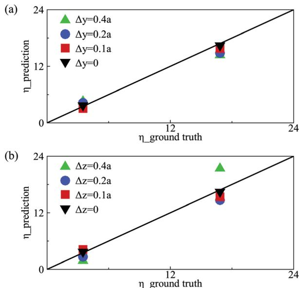
Fig. 8 Comparison of predicted membrane viscosity  $\eta$  with the corresponding ground truth for capsules with different initial off-centre distances along the (a) channel depth ( $y$ -direction), and (b) channel width ( $z$ -direction) at  $Ca = 0.6$ . The solid lines are guides for the eyes representing perfect agreement.
