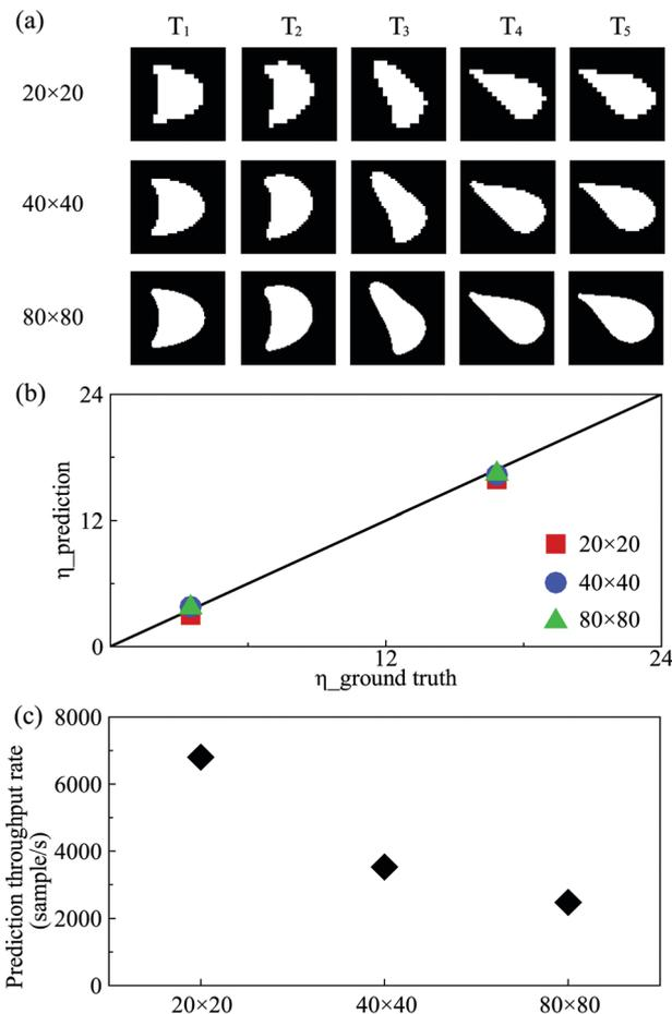
Fig. 7 (a) Binary images of capsule profiles with three resolutions. Comparisons of (b) predicted membrane viscosity  $\eta$  with the corresponding ground truth, and (c) prediction throughput rates of the DCNN-LSTM neural network using sample images with three different resolutions. The solid lines in (b) are guides for the eyes representing perfect agreement.
