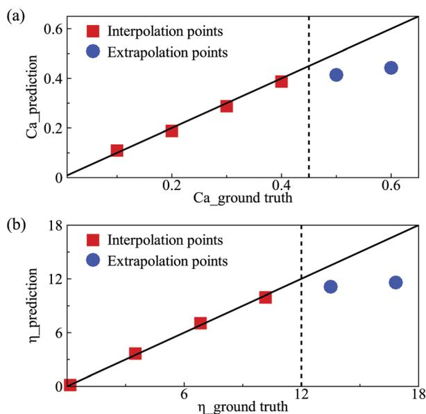
Fig. 9 Comparisons between the predicted (a) capillary number  $Ca$  (with  $\eta = 16.83$ ) and (b) membrane viscosity  $\eta$  (with  $Ca = 0.6$ ) and the corresponding ground truth. The solid lines are guides for the eyes representing perfect agreement. The dashed lines mark the parametric boundaries of the training samples.
