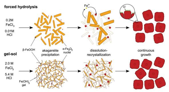
Fig. 2 Schematic representation of the formation mechanism of hematite cubes in the forced hydrolysis and gel-sol methods.
