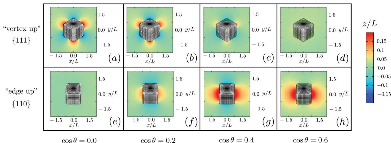
**Fig. 3** Contour plot of the deformation field induced by a single cube of side length  $L$  adsorbed at a fluid–fluid interface in the “vertex up”  $\{111\}$  and “edge up”  $\{110\}$  configuration, respectively, for the same Young contact angles  $\theta$  as in Fig. 2.
