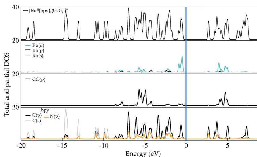
Fig. 2 Total and partial density (pDOS) for the starting complex  $[\text{Ru}(\text{bpy})_2(\text{CO})_2]^{2+}$ , also labeled as **1** in the text. Level of theory: PBE/500 eV, VASP code.<sup>57</sup> The fermi energy is set at zero.
