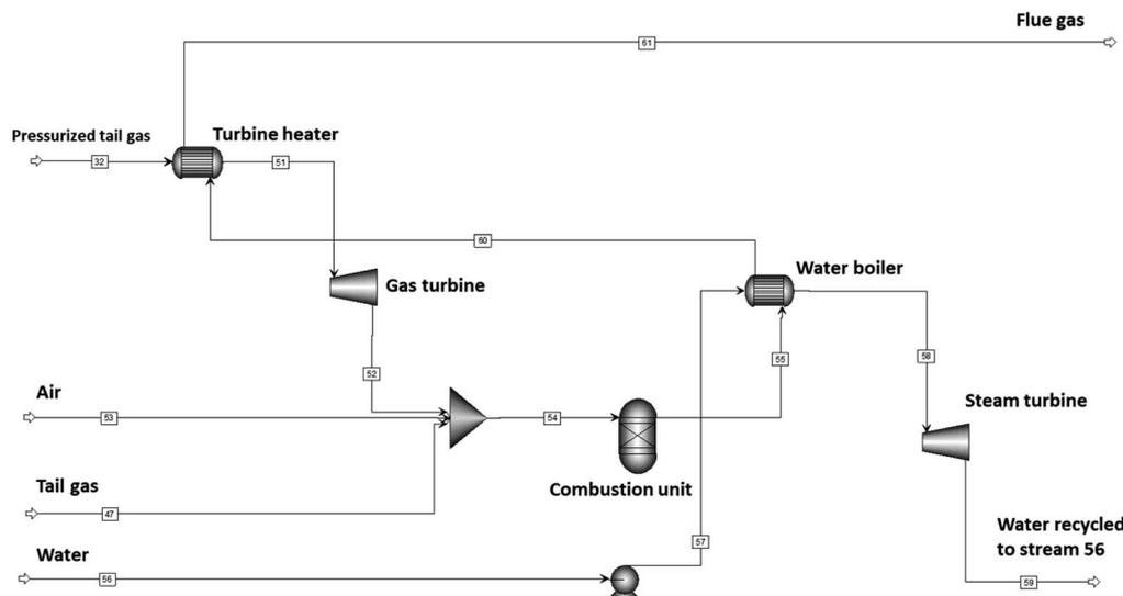
Fig. 6 Aspen model for the power plant.
