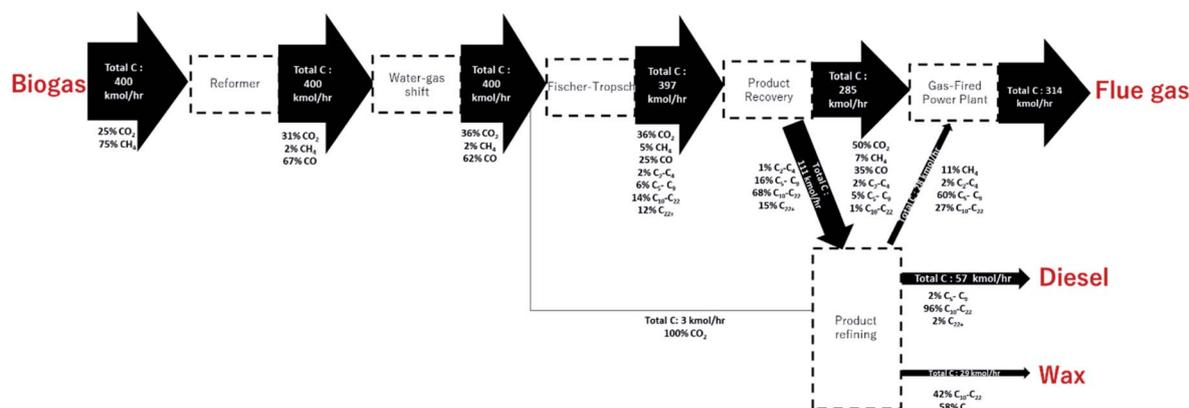
Fig. 7 Carbon flow diagram of the Fischer-Tropsch plant operating at  $X_{\text{CO}} = 60\%$  showing the distribution of carbon throughout the plant, including the distribution of carbon in (C-%) of different species in each section. Line thickness proportional to carbon flow.
