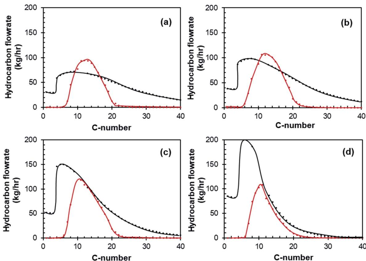
Fig. 11 Mass hydrocarbon distribution  $C_2$  to  $C_{40}$  product compounds for — Fischer-Tropsch products and — distillate product for  $X_{CO} =$  (a) 60%, (b) 70%, (c) 80% and (d) 90% for Pt-Co/ $Al_2O_3$  for the case with a hydrocracker.
