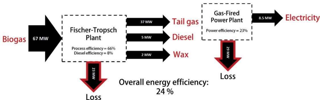
Fig. 8 Energy balance for base case design  $X_{\text{CO}} = 60\%$  for Pt–Co/ $\text{Al}_2\text{O}_3$  showing the lower heating values of reactants and products as well as the power generated from the plant.
