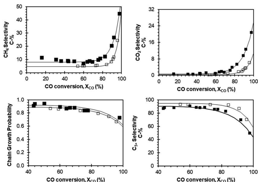
Fig. 4 Empirical modelling of the Fischer–Tropsch products as a function of conversion based on selectivity data from our previous study<sup>19,45</sup> for Pt–Co/Al<sub>2</sub>O<sub>3</sub> (closed symbols) and Mn–Pt–Co/Al<sub>2</sub>O<sub>3</sub> with a molar ratio of Mn : Co = 0.15 mol/mol (open symbols).
