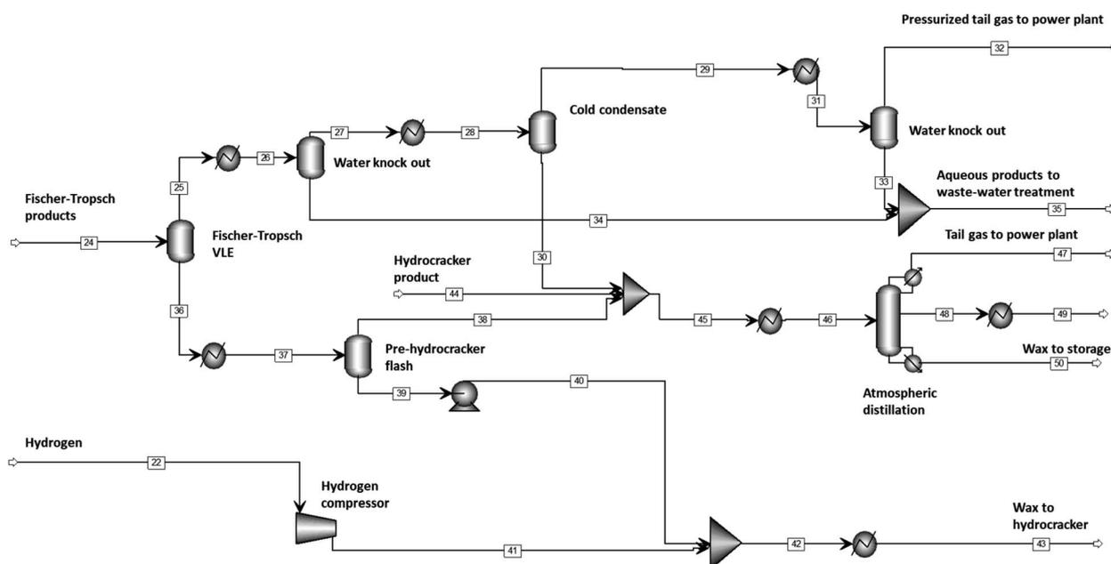
Fig. 5 Aspen model for Fischer–Tropsch product separation and distillate refining.
