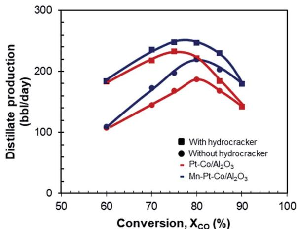
Fig. 12 Distillate production as a function of conversion for Pt–Co/Al<sub>2</sub>O<sub>3</sub> and Mn–Pt–Co/Al<sub>2</sub>O<sub>3</sub> with and without hydrocracking.
