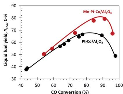
Fig. 2 The yield of  $\text{C}_{5+}$  as a function of CO conversion for standard industrial  $\text{Pt-Co/Al}_2\text{O}_3$  and industrial  $\text{Mn-Pt-Co/Al}_2\text{O}_3$  Mn : Co = 0.15 mol/mol.<sup>9,19</sup>
