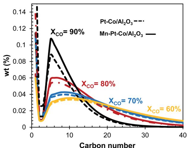
Fig. 9 Carbon number distribution for Pt–Co/ $\text{Al}_2\text{O}_3$  and Mn–Pt–Co/ $\text{Al}_2\text{O}_3$  in a slurry bed reactor at various conversions based on data from ref. 15 and 19.
