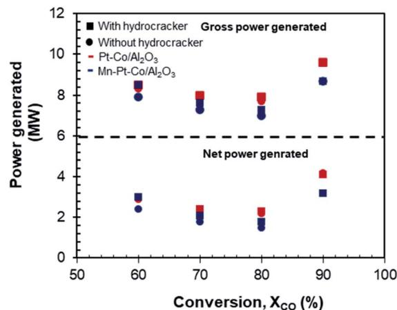
Fig. 13 Power generated as a function of conversion for Pt–Co/Al<sub>2</sub>O<sub>3</sub> and Mn–Pt–Co/Al<sub>2</sub>O<sub>3</sub> with and without hydrocracking.
