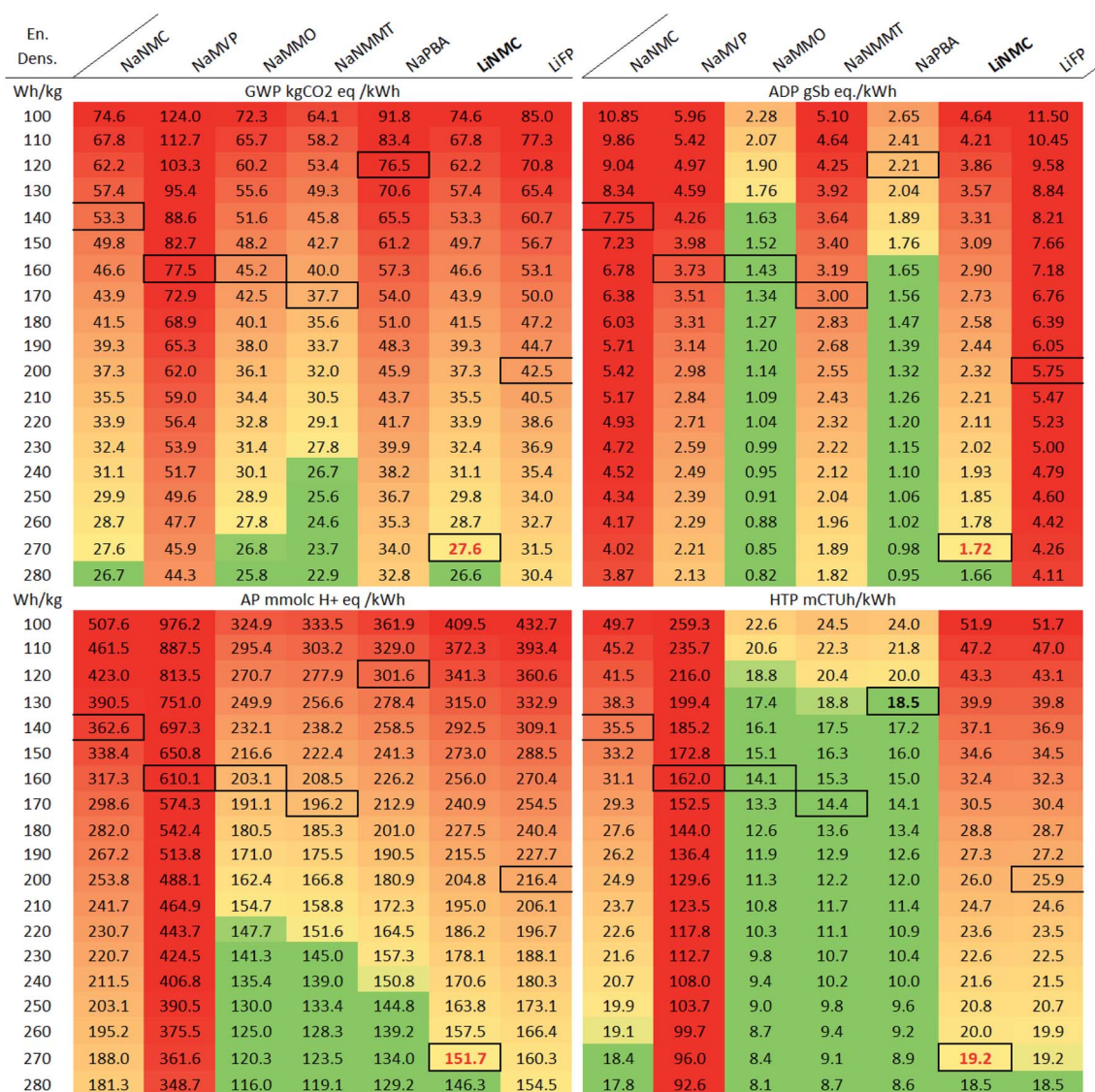
Fig. 4 Cradle-to-grave impacts per kWh of electricity provided by the battery cells over the lifetime of the assumed application for varying energy density, using PV electricity for charging. The thick frames mark the default values used in the assessment. The LiNC cell is used as common reference, and the colour coding indicates the performance relative to this benchmark (green colour: better than LiNC benchmark; yellow or red = worse). Moving the frame downwards until reaching the green area indicates the improvement in terms of cycle life required for equalling or excelling the benchmark cell (keeping all other parameters fixed).
