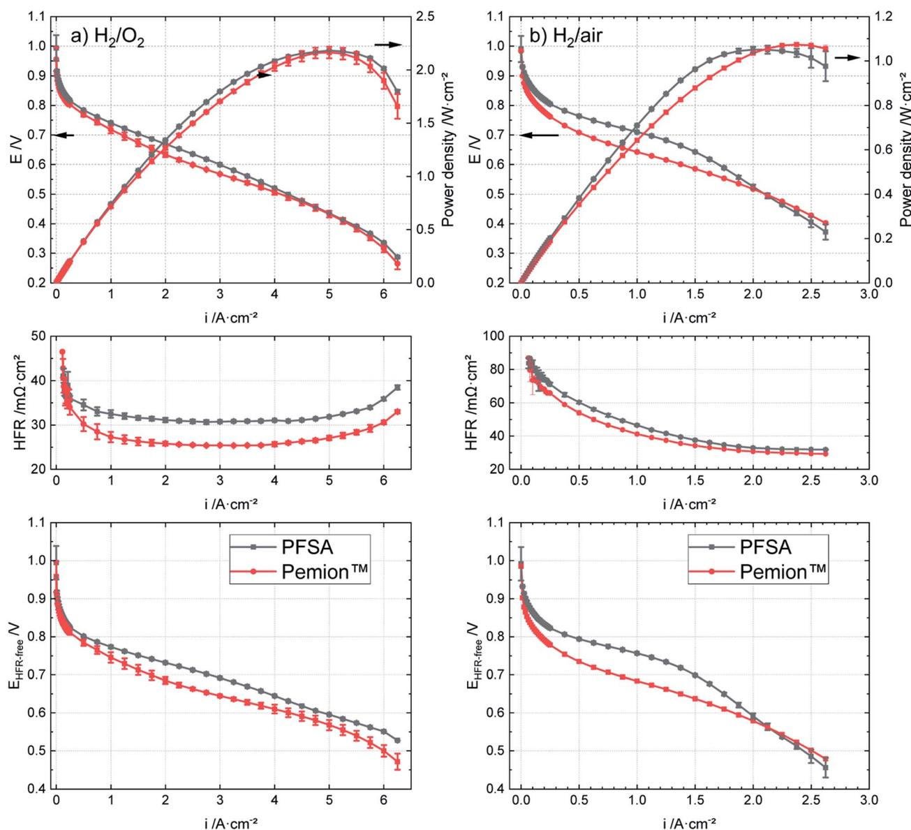
Fig. 2 Polarization behaviours, HFRs and HFR-corrected cell voltages of Pemion™ MEA vs. PFSA reference at 80 °C under (a)  $\text{H}_2/\text{O}_2$ , 0.25 slpm/1 slpm, 95% RH and ambient pressure and (b)  $\text{H}_2/\text{air}$ , 0.25 slpm/1 slpm, 50% RH, 250  $\text{kPa}_{\text{abs}}$ .
