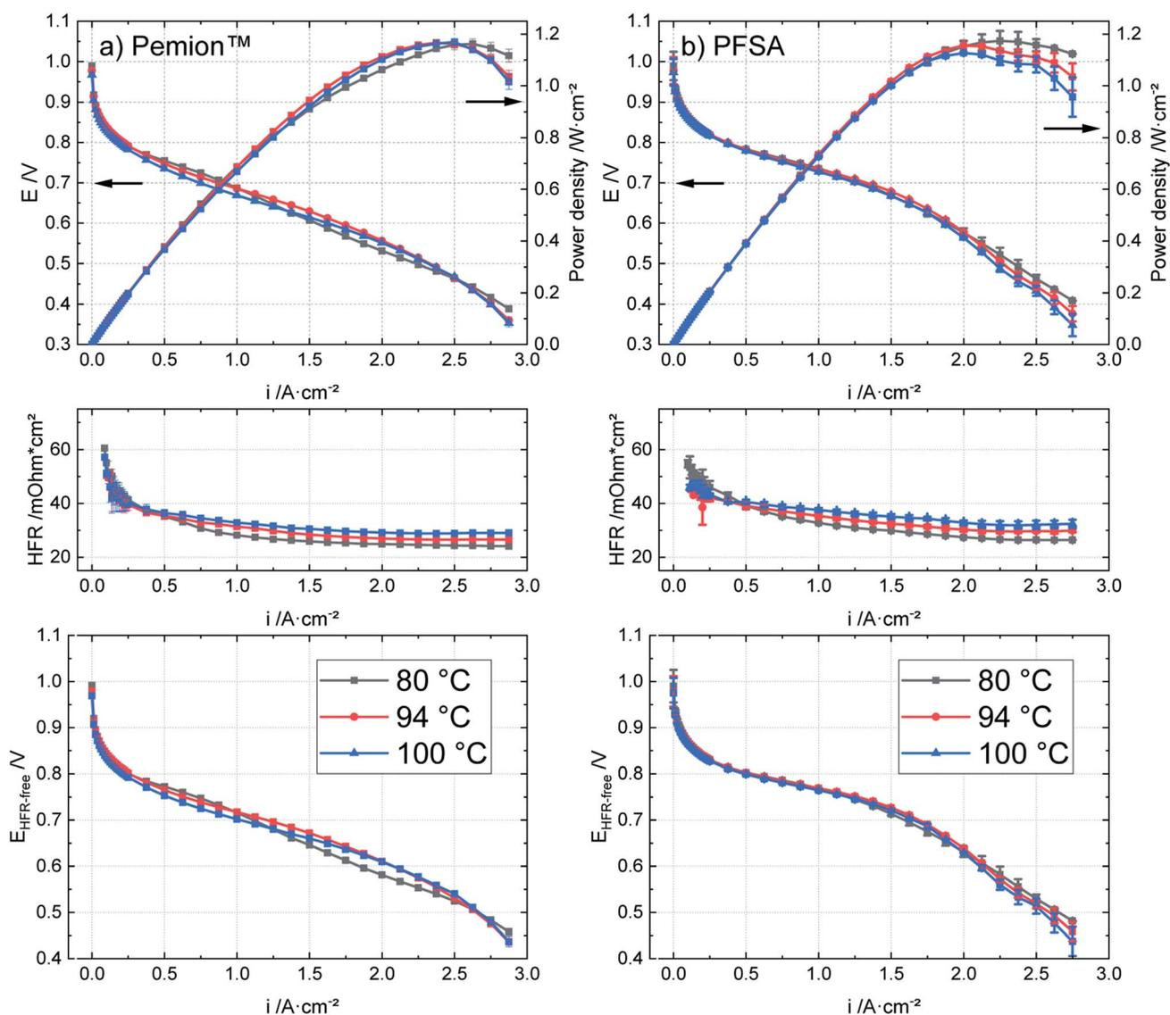
Fig. 6 Polarization behaviours, HFR and HFR-corrected cell voltages of (a) Pemion™ MEA and (b) PFSA reference MEA under 80 °C, 94 °C and 100 °C at 80% humidified  $\text{H}_2/\text{air}$ , 250  $\text{kPa}_{\text{abs}}$ .
