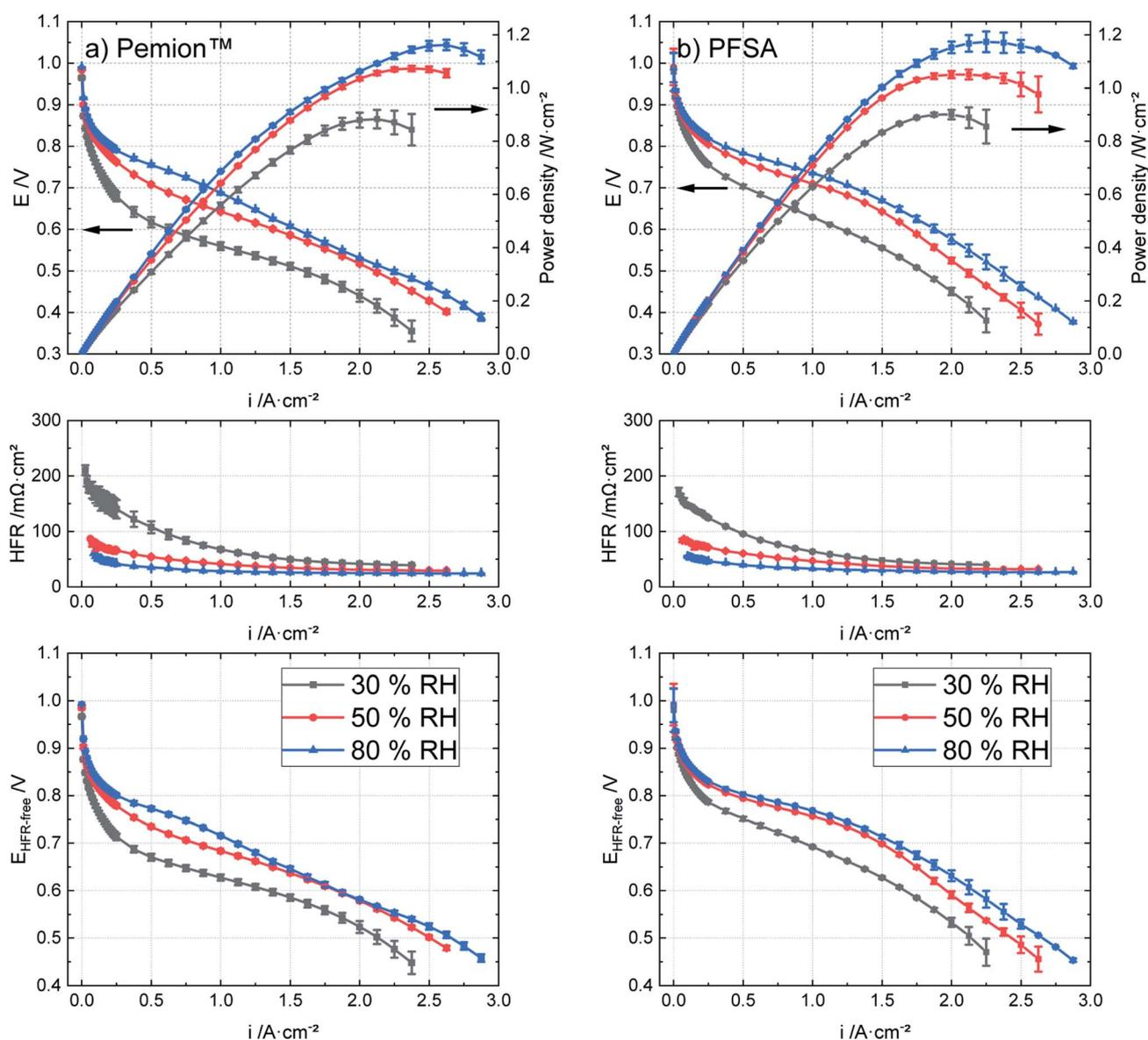
**Fig. 4** Polarization behaviours, HFR and HFR-corrected cell voltages of (a) Pemion™ MEA and (b) PFSA reference under varied RH levels at 80 °C, H<sub>2</sub>/air, 250 kPa<sub>abs</sub>.
