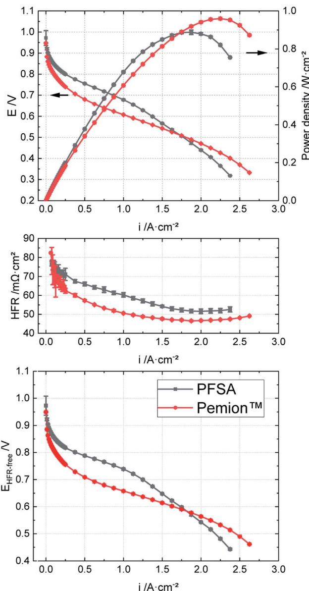
Fig. 8 Polarization behaviours, HFR and HFR-corrected cell voltages of Pemion™ MEA vs. PFSA reference at 110 °C under H<sub>2</sub>/air, 50% RH, 250 kPa<sub>abs</sub>.
