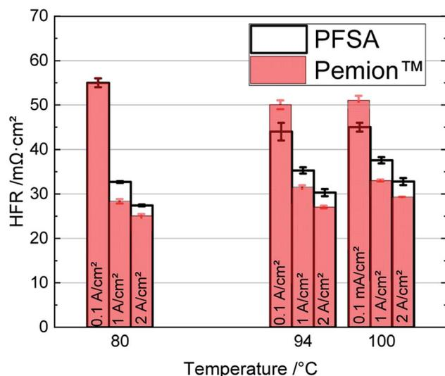
Fig. 7 Direct comparison of the HFRs of Pemion™ MEA and PFSA reference MEA at different current densities (0.1 A cm<sup>-2</sup>, 1 A cm<sup>-2</sup>, 2 A cm<sup>-2</sup>) under operating temperatures 80 °C, 94 °C, and 100 °C.
