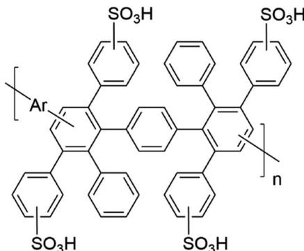
Fig. 1 Structures of Pemion™ – a variation of sulfo-phenylated polyphenylenes (sPPX-H<sup>+</sup>).
