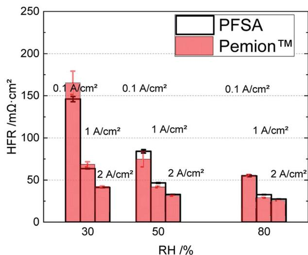
Fig. 5 Direct comparison of the HFRs of Pemion™ MEA and PFSA reference MEA at different current densities (0.1 A cm<sup>-2</sup>, 1 A cm<sup>-2</sup> and 2 A cm<sup>-2</sup>) under varied RH levels (30%, 50% and 80%).
