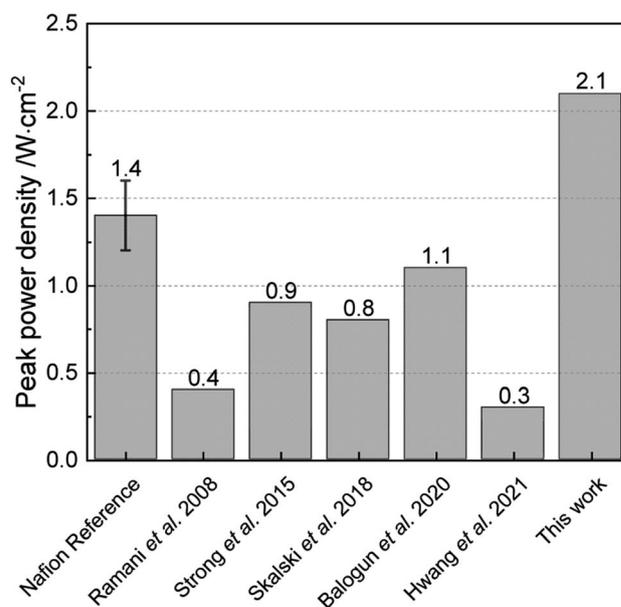
Fig. 3 Peak power densities of fully hydrocarbon MEAs over the last decades under the same conditions: 80 °C, H<sub>2</sub>/O<sub>2</sub>, high humidity (>75% RH) and ambient pressure.<sup>33–36,47</sup>
