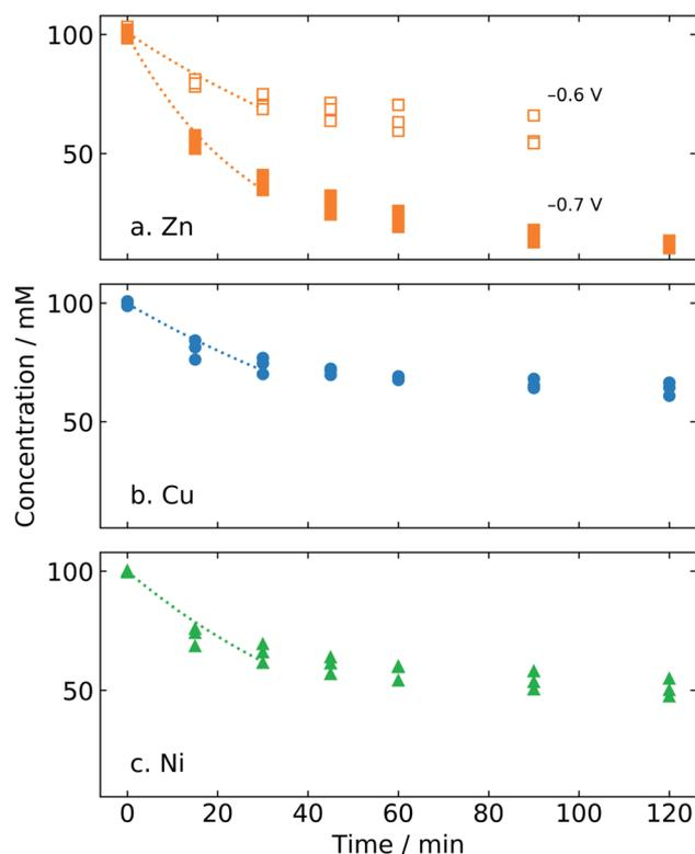
Fig. 8 Experimental furfural concentration profiles during electrolysis in 0.5 M NaHCO<sub>3</sub> with the (a) zinc catalyst at  $-0.6$  and  $-0.7$  V vs. RHE; (b) copper catalyst at  $-0.7$  V vs. RHE; (c) nickel catalyst at  $-0.7$  V vs. RHE. Curves represent fitting of the initial reaction rate (0–30 min) to a first order rate law.
