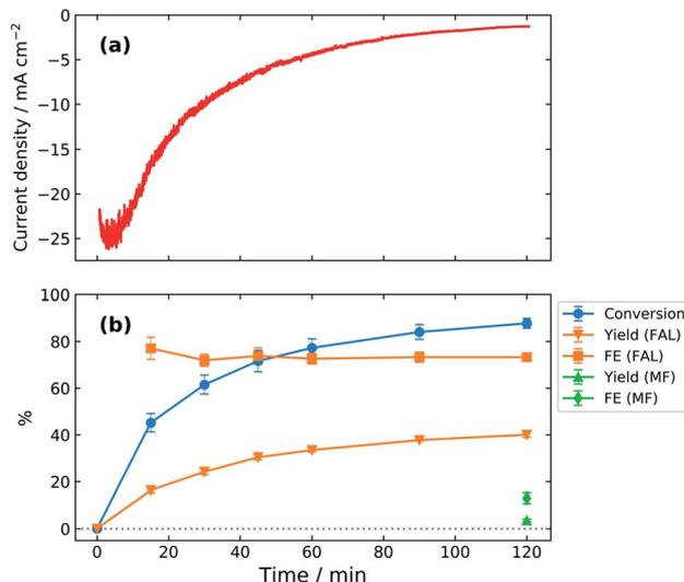
Fig. 3 Potentiostatic electrolysis of furfural on the zinc catalyst in 0.5 M NaHCO<sub>3</sub> at -0.7 V vs. RHE (a) chronoamperometry during electrolysis; (b) evolution of the conversion, yield, and FE of products.
