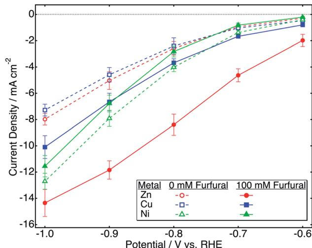
Fig. 2 Furfural reduction and HER polarization curves obtained with different catalysts in 0.5 M NaHCO<sub>3</sub>.
