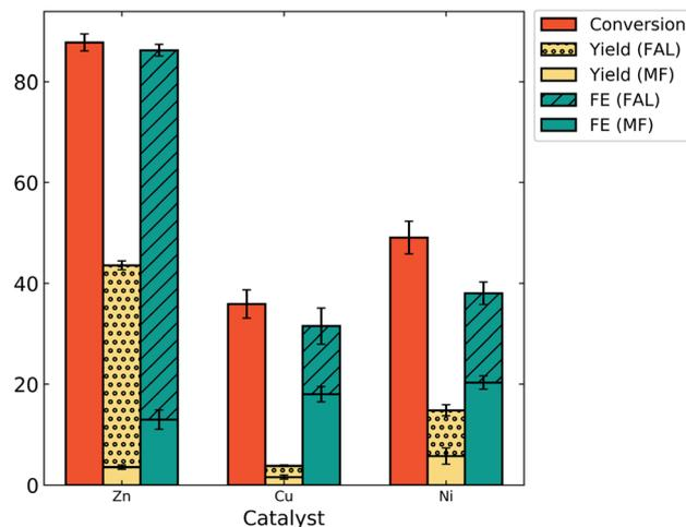
Fig. 6 ECH electrolysis results with different catalysts in 0.5 M NaHCO<sub>3</sub> at −0.7 V vs. RHE.
