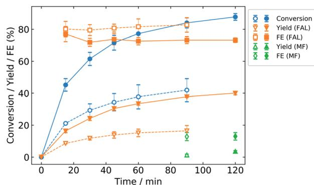
Fig. 5 ECH electrolysis results with the zinc catalyst in 0.5 M NaHCO<sub>3</sub> at different cathode potentials. Open symbols with dashed lines:  $-0.6$  V vs. RHE. Closed symbols with solid lines:  $-0.7$  V vs. RHE.
