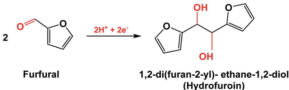
Scheme 2 Electrodimerization reaction of furfural to hydrofuroin.<sup>33</sup>
