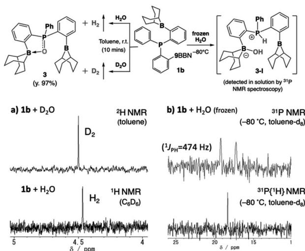
Fig. 2 Reaction schemes and NMR spectra of **1b** with  $\text{H}_2\text{O}$  and  $\text{D}_2\text{O}$  at room temperature (a) and with frozen water at –80 °C (b).
