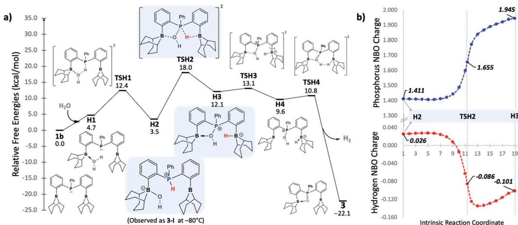
Fig. 3 Proposed reaction mechanism for the formation of 3 calculated at the SMD(benzene):  $\omega$ -B97XD/6-311G(d) level (298 K) (a) and NBO charges of the phosphorus and transfer of hydrogen atoms from H2 (observed in the NMR spectrum as 3-I) to H3 (b).
