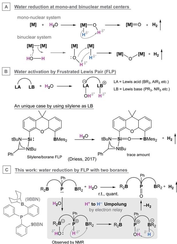
Chart 1 Metal- (A) and p-block element (B and C)-based mechanisms for water activation and reduction.
