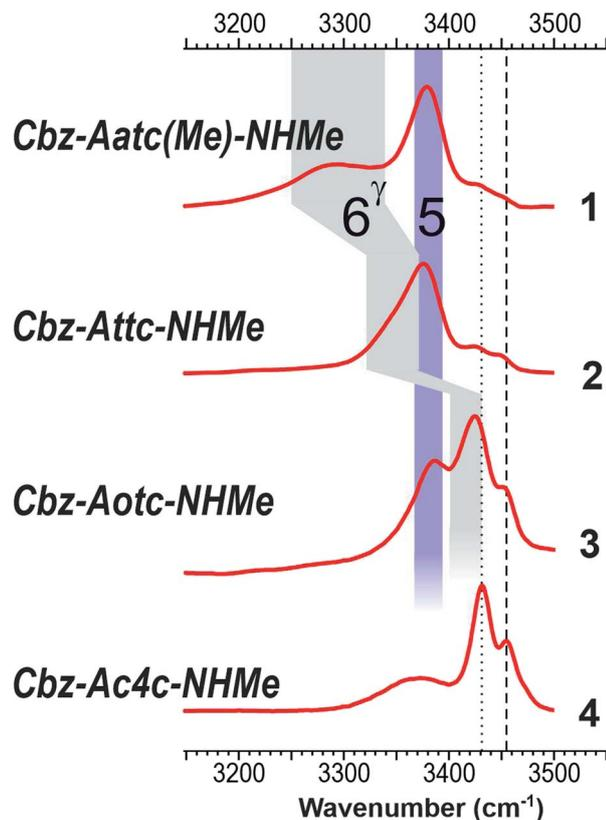
Fig. 5 Chloroform solution IR spectra of compounds 1–4, with highlighted C5 (violet) and C6 $\gamma$  (grey) spectral regions. Bands assigned to free NH(1) and NH(2) vibrators are marked as dotted and dashed lines respectively.
