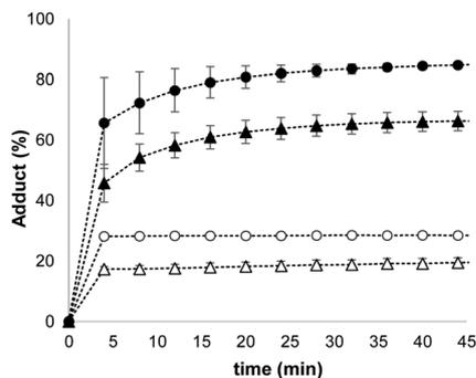
Fig. 5 Time course for conversion of **2** (50  $\mu\text{M}$ ) embedded in vesicles (DOPC, 0.5 mM in HEPES buffer at pH 7.2) into the corresponding Michael adduct on addition of different thiols: 100  $\mu\text{M}$  benzyl thiol (▲), 200  $\mu\text{M}$  benzyl thiol (●), 5.0 mM 2-mercaptoethanesulfonate (Δ), 10 mM 2-mercaptoethanesulfonate (○).
