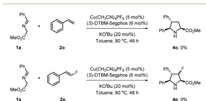
Scheme 3 Reactions of styrene **2o** and monofluorostyrene **2p**.
