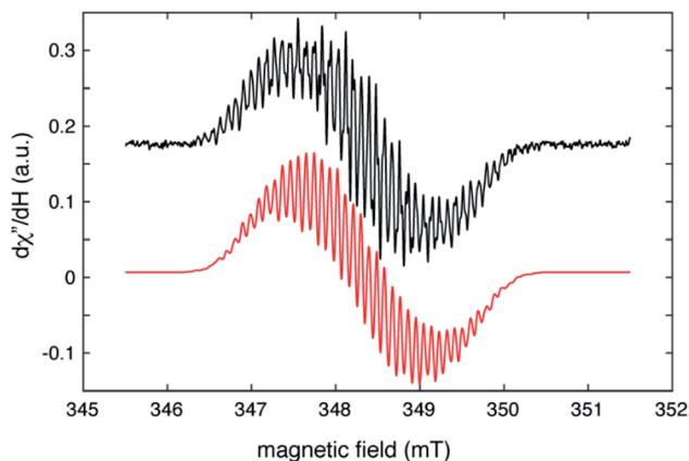
Fig. 5 Cw-EPR spectrum of  $(Cp^{Me4H})_2Y(abpy')$ , **1** (black trace), collected under the following conditions: microwave frequency, 9.7788 GHz; microwave power, 80  $\mu$ W; modulation amplitude, 0.02 mT, modulation frequency, 100 KHz; sample temperature, 295 K. The red trace is a simulation produced by using the isotropic hyperfine couplings and model described in the text and summarized in Table 1.
