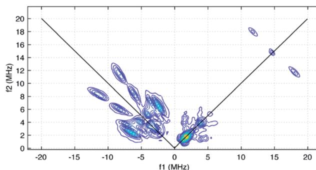
Fig. 6 HYSCORE spectrum of  $(Cp^{Me4H})_2Y(abpy')$ , **1**, taken under the following conditions: microwave frequency, 9.7405 GHz; magnetic field, 347.0 mT;  $\tau$ -value, 204 ns; sample temperature, 40 K. Data are displayed using a threshold of 5% of the maximum peak amplitude.
