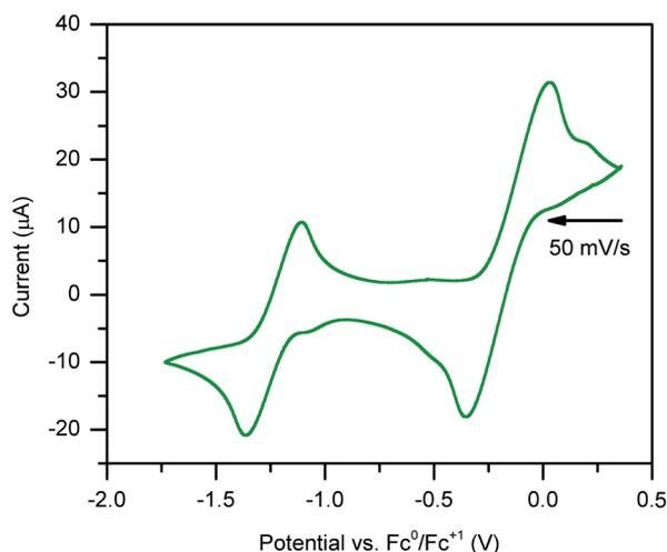
Fig. 8 Cyclic voltammogram of (Cp<sup>Me4H</sup>)<sub>2</sub>Y(abpy<sup>•-</sup>) vs. Fc. 250 mM [N<sup>n</sup>Bu<sub>4</sub>][PF<sub>6</sub>] in THF and 3 mM analyte. Voltammogram features two quasi-reversible redox events: one process at  $E_{1/2} = -1.2 \pm 0.244$  V, and one irreversible process at approximately  $-0.2 \pm 0.244$  mV.
