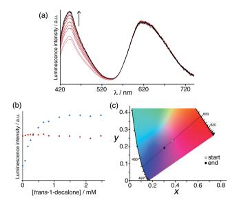
Fig. 7 Results of titration of the cavity-binding guest trans-1-decalone into a combination of  $H^W$  (150  $\mu$ M), MAC (10  $\mu$ M) and Ru (50  $\mu$ M) in water. (a) Fluorescence changes associated with MAC being displaced from the cage cavity ( $\lambda_{exc} = 395$  nm); (b) plot of the peak intensity data from part (a) during the titration; (c) shift in overall emission colour on a CIE colour-space chart during the titration.
