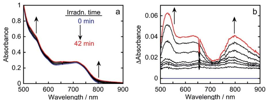
Fig. 6 (a) Absorption spectral changes of a CO<sub>2</sub>-saturated DMA solution containing Os (0.1 mM) and BI(OH)H (0.2 M) during irradiation at 480 nm with a light intensity of  $2.6 \times 10^{-8}$  einstein s<sup>-1</sup> (0–42 min at 6 min intervals) and (b) difference spectra from post- and pre-irradiation spectra. The blue and red lines represent the spectra before irradiation and after irradiation for 42 min, respectively.
