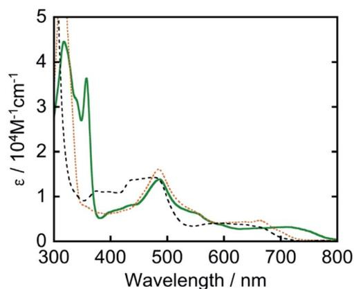
Fig. 1 UV-vis absorption spectrum of **Os** (green solid line) measured in DMA along with those of  $[\text{Os}(\text{5dmb})_2(\text{dmb})]^{2+}$  in *N,N*-dimethylformamide (black broken line) and  $[\text{Os}(\text{mtpy})_2]^{2+}$  in DMA (orange dashed line).
