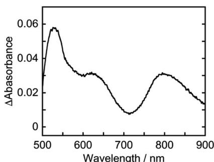
Fig. 7 Difference absorption spectrum from before and after electrolytic one-electron reduction of Os. A CO<sub>2</sub>-saturated DMA solution containing Os (0.5 mM) and Et<sub>4</sub>NBF<sub>4</sub> (0.1 M) as an electrolyte was reduced at -1.75 V using a UV-vis OTTLE cell with a Pt mesh working electrode and Ag/AgNO<sub>3</sub> reference electrode.
