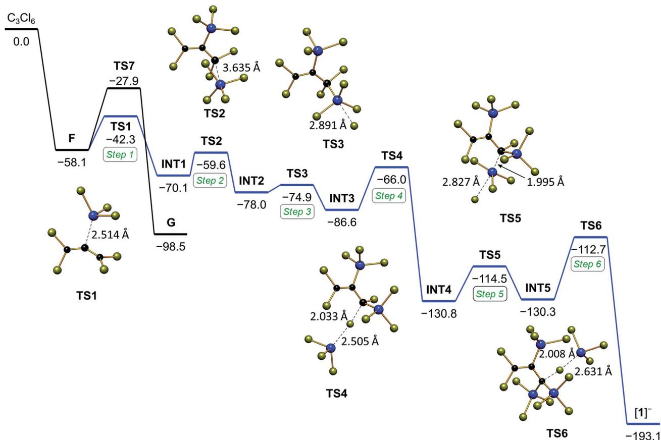
**Scheme 3** Top: reaction of  $C_3Cl_6$  with  $Si_2Cl_6$  and  $Cl^-$  furnishes perchloroallene **F**, which can either dimerize to **G** (black pathway) or react further to  $[1]^-$  (blue pathway). Bottom: Gibbs free energy ( $\text{kcal mol}^{-1}$ ) diagram for the formation of  $[1]^-$  computed at the  $\omega B97X-D3(BJ)/ma-def2-QZVPP+COSMO-RS//ma-def2-TZVP(CPCM(CH_2Cl_2))$  level of theory (standard conditions).
