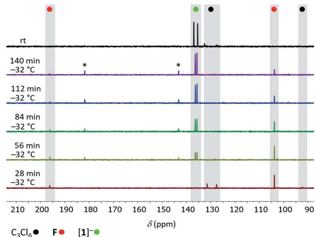
Fig. 2  $^{13}\text{C}\{^1\text{H}\}$  NMR spectra recorded at  $-32\text{ }^\circ\text{C}$  at 28 min intervals on the reaction mixture  $\text{C}_3\text{Cl}_6 : \text{Si}_2\text{Cl}_6 : [\text{nBu}_4\text{N}]\text{Cl}$  (1 : 4 : 1;  $\text{CD}_2\text{Cl}_2$ ) and at room temperature (top); (\*) unknown intermediate.
