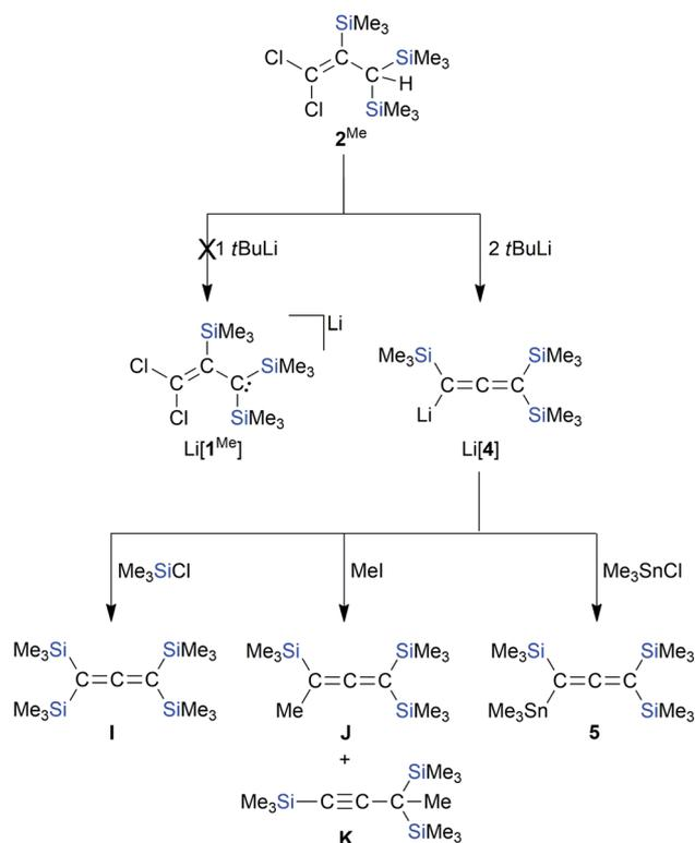
**Scheme 5** The reaction of  $2^{\text{Me}}$  with *t*BuLi does not lead to  $\text{Li}[1^{\text{Me}}]$  but to **Li[4]**. **Li[4]** reacts with  $\text{Me}_3\text{SiCl}$ , MeI, or  $\text{Me}_3\text{SnCl}$  to form the derivatives **I**, **J/K**, or **5**, respectively (THF, room temperature).
