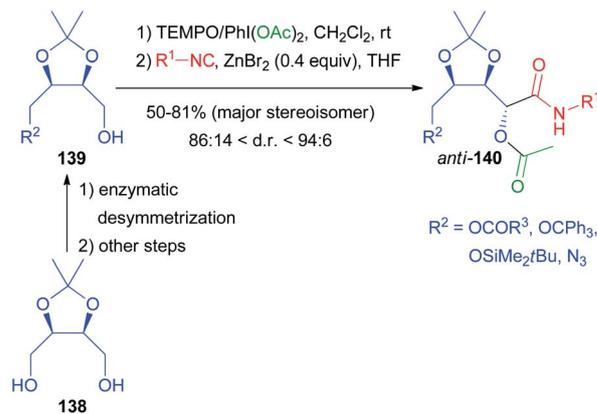
Scheme 40 Diastereoselective Passerini reaction catalysed by ZnBr<sub>2</sub>.
