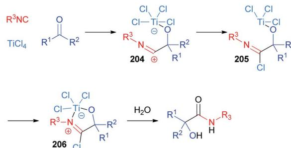
Scheme 55 Mechanism of the TiCl<sub>4</sub> mediated Passerini reaction.
