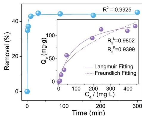
Fig. 4 Removal percentage of  $\text{IO}_3^-$  as a function of contact time fitted with the pseudo-second-order kinetic model. Inset: adsorption isotherms of  $\text{IO}_3^-$  by **Th-SINAP-200** fitted with the Langmuir model and the Freundlich model.
