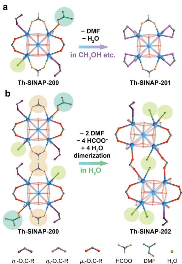
Fig. 2 Schematic diagrams showing the evolution of coordination environments of  $\text{Th}_6(\mu_3\text{-OH})_8$  SBUs (a) from **Th-SINAP-200** to **Th-SINAP-201** and (b) from **Th-SINAP-200** to **Th-SINAP-202**. Only the coordination environments on the equatorial planes are shown and eight  $\text{TCBPA}^{3-}$  ligands are omitted for clarity.
