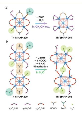
Fig. 2 Schematic diagrams showing the evolution of coordination environments of  $Th_6(\mu_3-OH)_8$  SBUs (a) from Th-SINAP-200 to Th-SINAP-201 and (b) from Th-SINAP-200 to Th-SINAP-202. Only the coordination environments on the equatorial planes are shown and eight TCBPA<sup>3-</sup> ligands are omitted for clarity.
