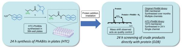
Fig. 1 (a) Schematic representation of previous work describing the PhotoAffinity Bit (PhABit) screening technology. (b) D2B-HTC PhABit screening platform. PhABits can be synthesised in 384-well plates in 24 h and screened as crude reaction products with a protein target.
