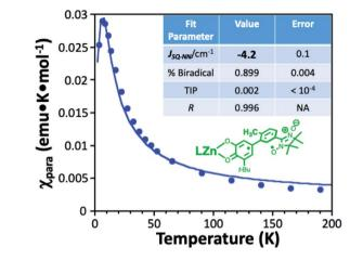
Fig. 3 Variable-temperature paramagnetic susceptibility data for LZn(SQ-6-Me-mPh-NN) (L = hydro-tris(cumenyl, methyl-pyrazolyl) borate), see ESI† for details. The best fit of eqn (2) to the data yields  $J_{\text{SQ-NN}} = -4 \text{ cm}^{-1}$ .
