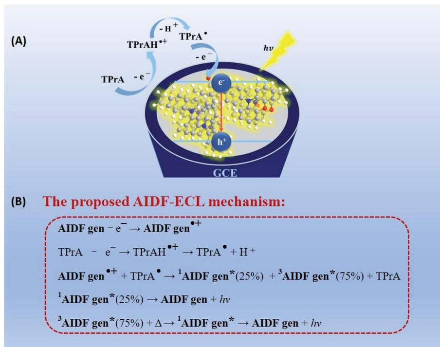
Fig. 3 (A) The schematic subprocesses of oxidative-reduction ECL of the AIDF-luminogen-modified GCE/TPrA couple and (B) the proposed ECL mechanisms, in which  ${}^1\text{AIDF gen}^*$  and  ${}^3\text{AIDF gen}^*$  represent singlet and triplet excited states that were electrochemically generated on AIDF luminogens, respectively.
