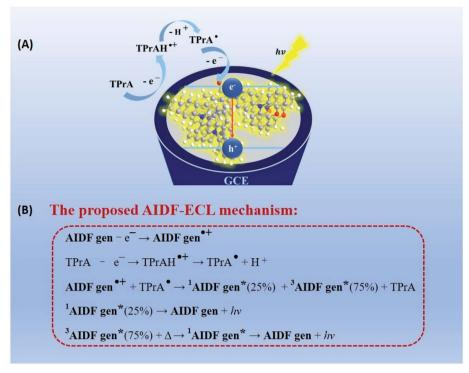
Fig. 3 (A) The schematic subprocesses of oxidative-reduction ECL of the AIDF-luminogen-modified GCE/TPrA couple and (B) the proposed ECL mechanisms, in which 1AIDF gen\* and 3AIDF gen\* represent singlet and triplet excited states that were electrochemically generated on AIDF luminogens, respectively.
