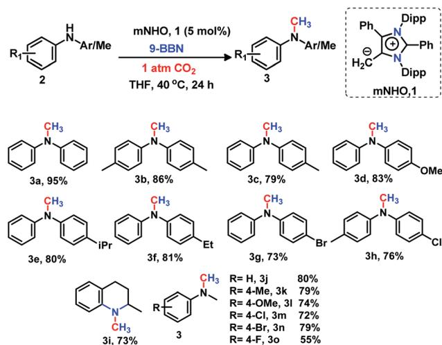
Scheme 2 mNHO catalysed *N*-methylation of secondary amines. Reaction conditions: amines (0.2 mmol), CO<sub>2</sub> (1 atm), 9-BBN (0.8 mmol), and dry THF (0.5 mL). Isolated yields (average yield of two catalytic runs) are reported.
