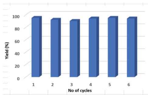
**Scheme 3** Longevity of the catalyst. Reaction conditions: amines (0.2 mmol), CO<sub>2</sub> (1 atm), 9-BBN (0.8 mmol), and dry THF (0.5 mL). A bar diagram showing yield (average yield of two experiments) versus number of catalytic cycles, emphasizing that the catalyst remains equally efficient over six successive catalytic cycles.
