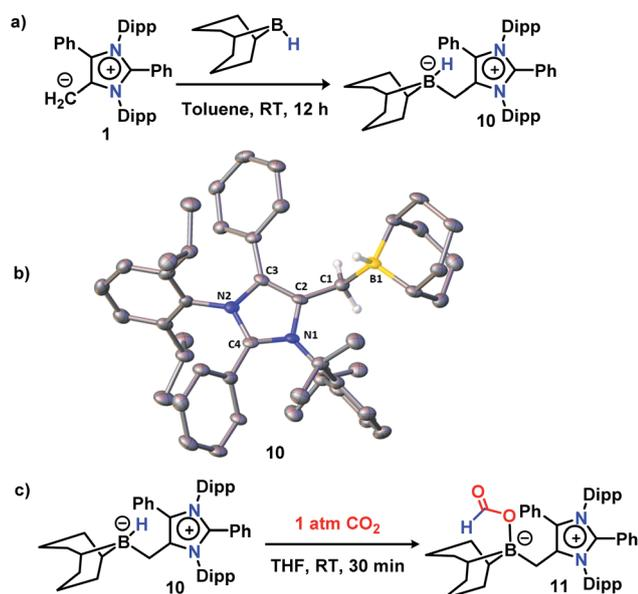
**Fig. 1** (a) Stoichiometric reaction between mNHO **1** and 9-BBN resulting in the formation of **10**. (b) The X-ray structure of **10**. Ellipsoids are set at the 50% probability level; hydrogen atoms except  $-\text{CH}_2$  and the B–H hydrogens have been omitted for the sake of clarity. (c) A control reaction between **10** and CO<sub>2</sub> reveals the formation of mNHO–boron formate **11** via insertion of CO<sub>2</sub> into the activated B–H bond.
