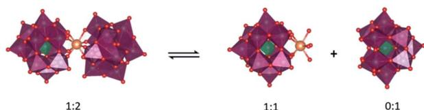
Fig. 1 Equilibrium between Ce<sup>IV</sup>K 1 : 2 ([Ce<sup>IV</sup>( $\alpha$ -PW<sub>11</sub>O<sub>39</sub>)<sub>2</sub>]<sup>10-</sup>) and Ce<sup>IV</sup>K 1 : 1 ([Ce<sup>IV</sup>( $\alpha$ -PW<sub>11</sub>O<sub>39</sub>)]<sup>3-</sup>). Color code: Ce – golden sphere; O – red spheres; {WO<sub>6</sub>} – purple octahedra; {PO<sub>4</sub>} – green tetrahedra. Ce<sup>IV</sup>K (1 : 1) could coordinate to oxygens from water, peptides, or proteins.
