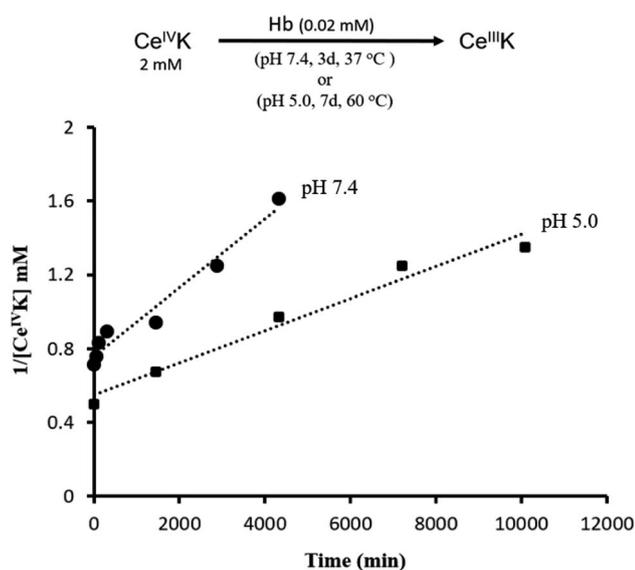
Fig. 3 Plot of  $1/[\text{Ce}^{\text{IV}}\text{K}]$  (mM) versus time (min) in the presence of Hb, at pH 7.4 and 37 °C, and pH 5.0 and 60 °C, showing second order kinetic in  $\text{Ce}^{\text{IV}}\text{K}$ .
